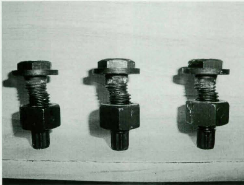
Test 3A – Connection Bolts at End of Test (fit back together)
