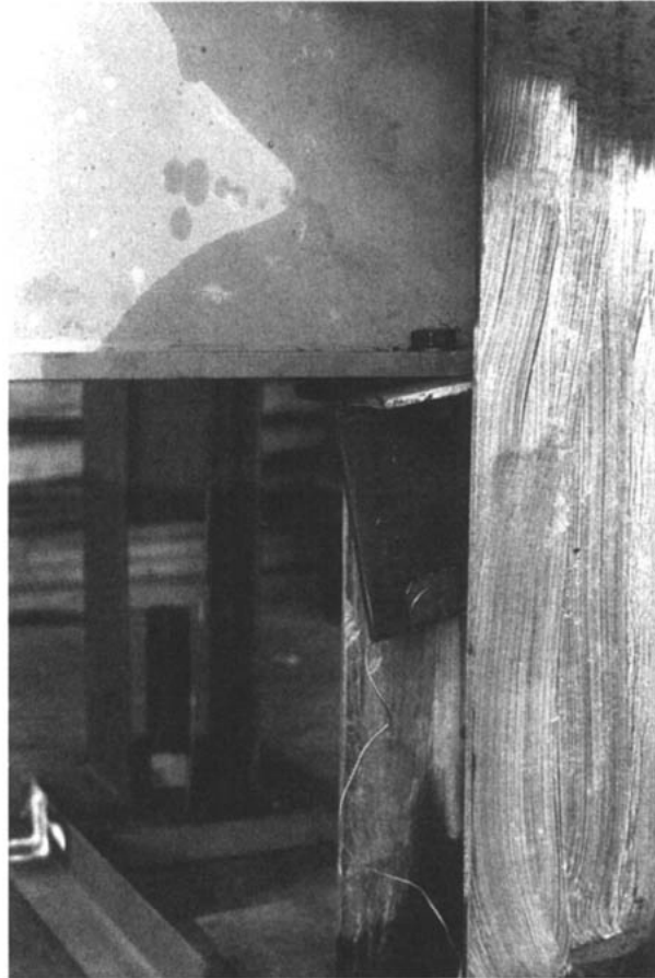
Figure 1. Column Web Rotation at Ultimate Load
