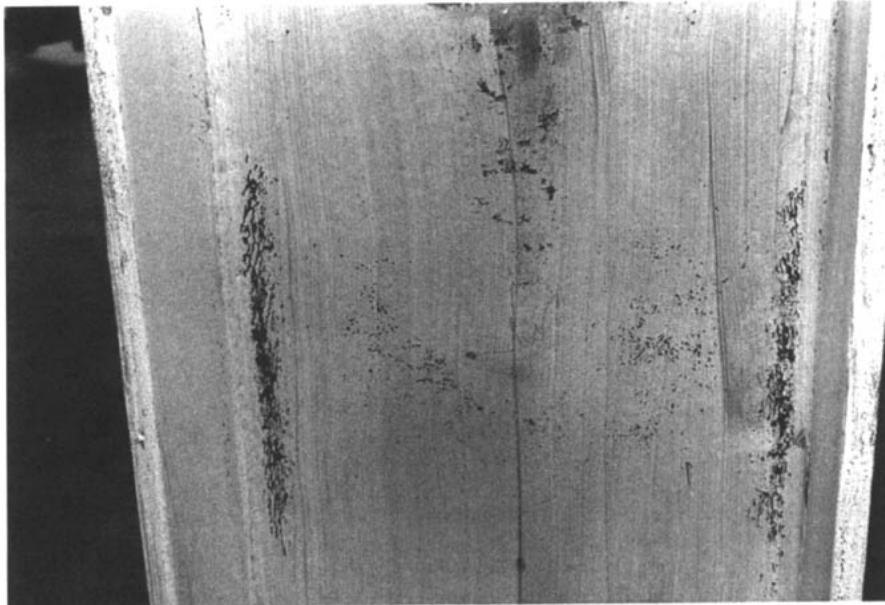
Figure 4. Development of Yield Line Mechanism
