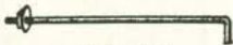
Fig. 145 Standard Wall Plate Bolt. \frac{5}{8} " \phi —2'-6" lg. turned 3" one end. Cut washer and nut other end.
