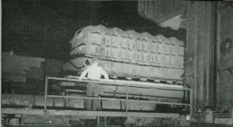
Box Annealing at the Inland Steel Company—Sealed material is shown being rolled into annealing furnace.
