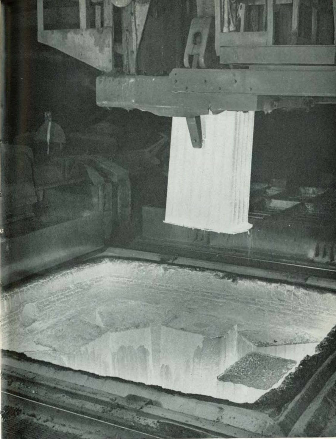
Ingots lose some of their heat after they leave the open hearth building so are reheated in soaking pits to a rolling temperature of approximately 2400° F.
