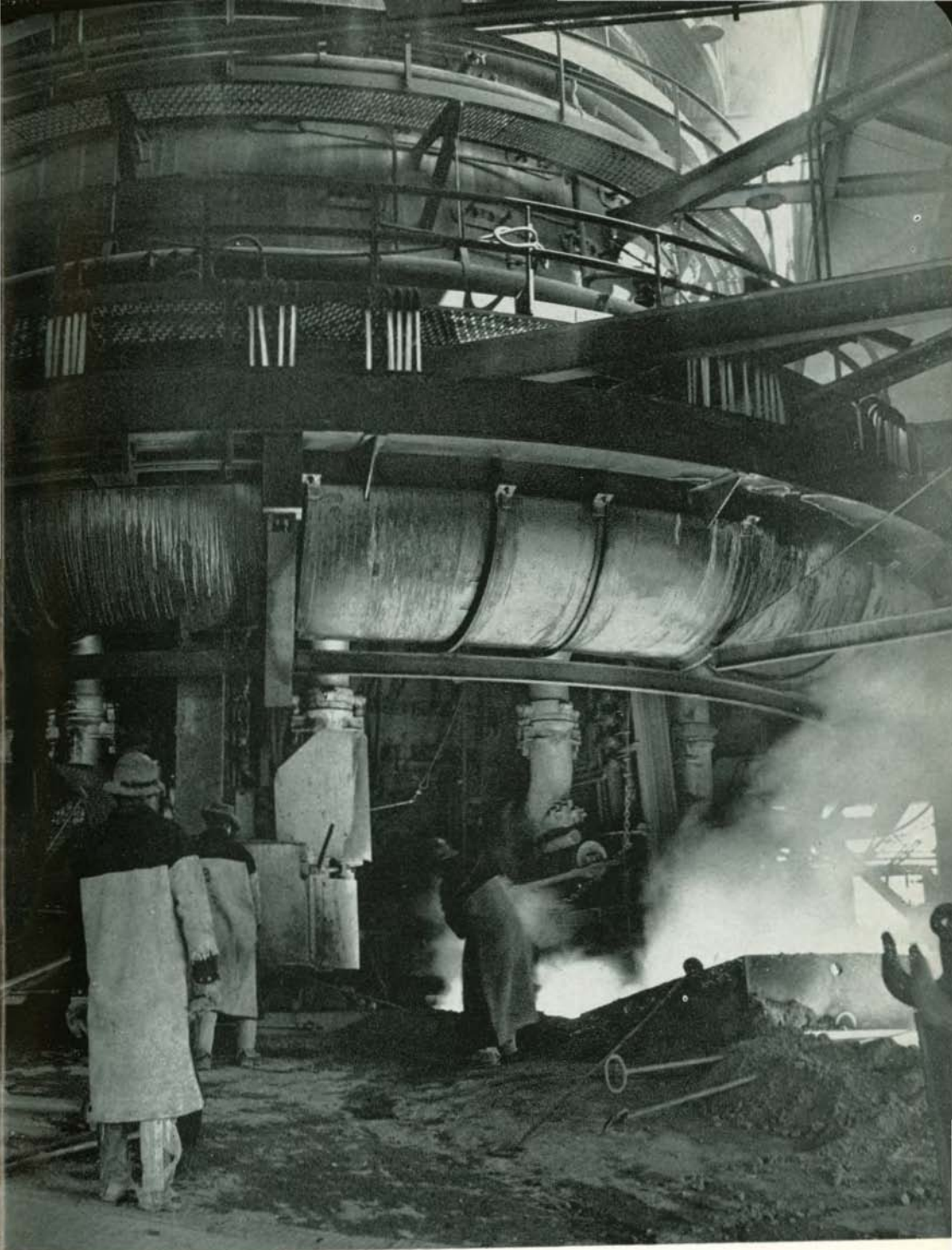
On the casting floor of a Kaiser Steel blast furnace 250 tons of pig iron are drawn off every five hours. Three furnaces are in operation.
