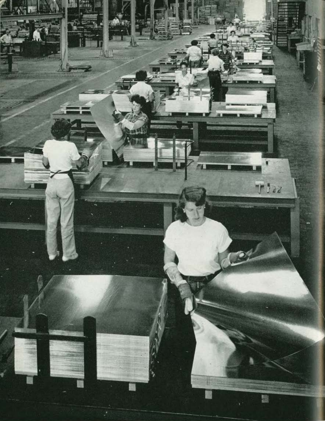
As the final step before packaging, each sheet of finished tin plate is individually inspected on both sides by women who wear heavy gloves to protect their hands.
