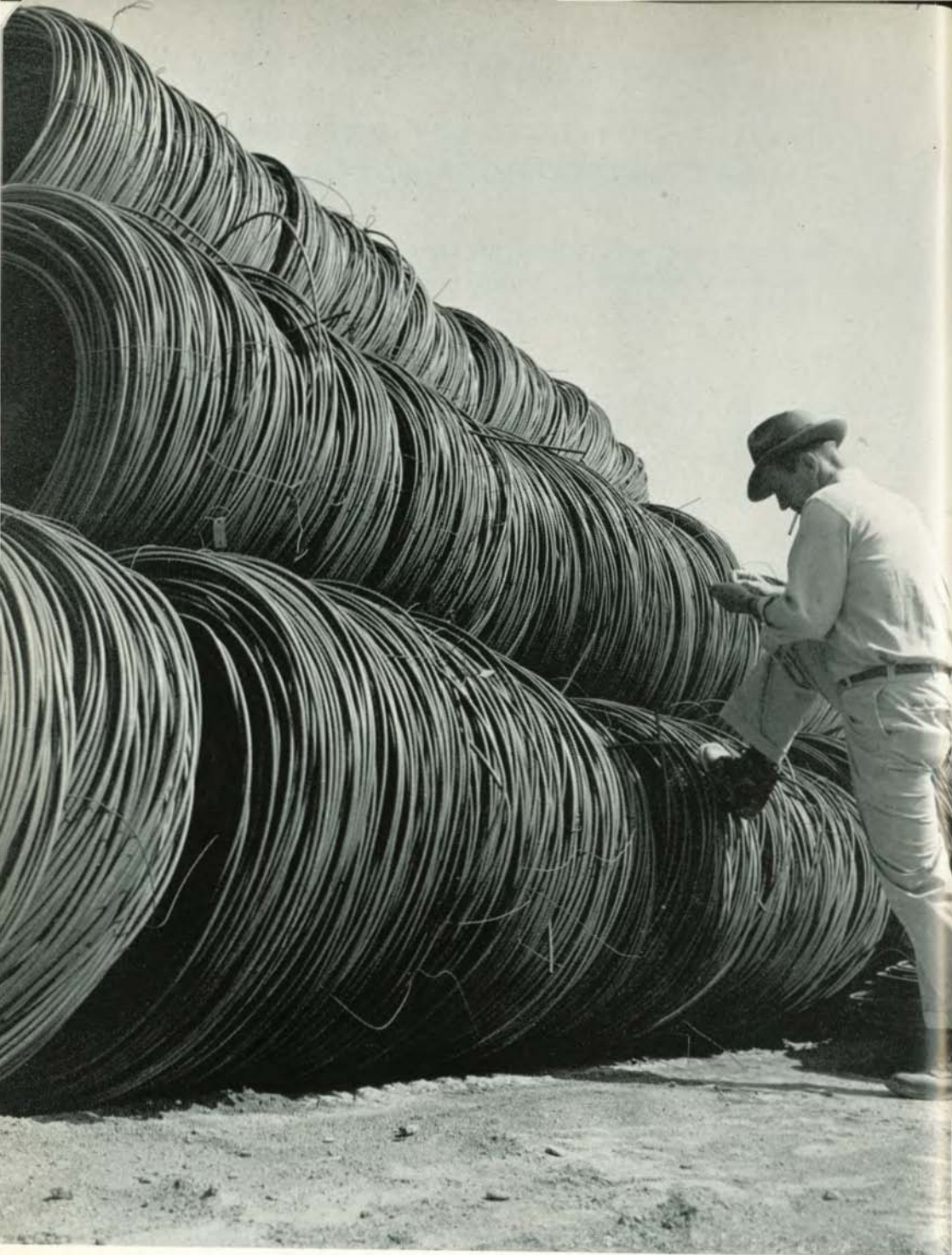
Coiled rods are rolled in continuous lengths from double converted billets on a combination mill.
