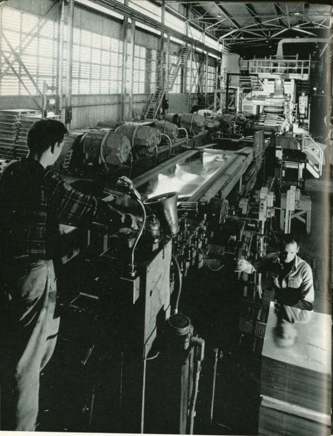
At the exit end of the electrolytic line, tin plate is sheared, inspected, sorted and stacked. Electrolytic tinning requires less tin than hot dip method.
