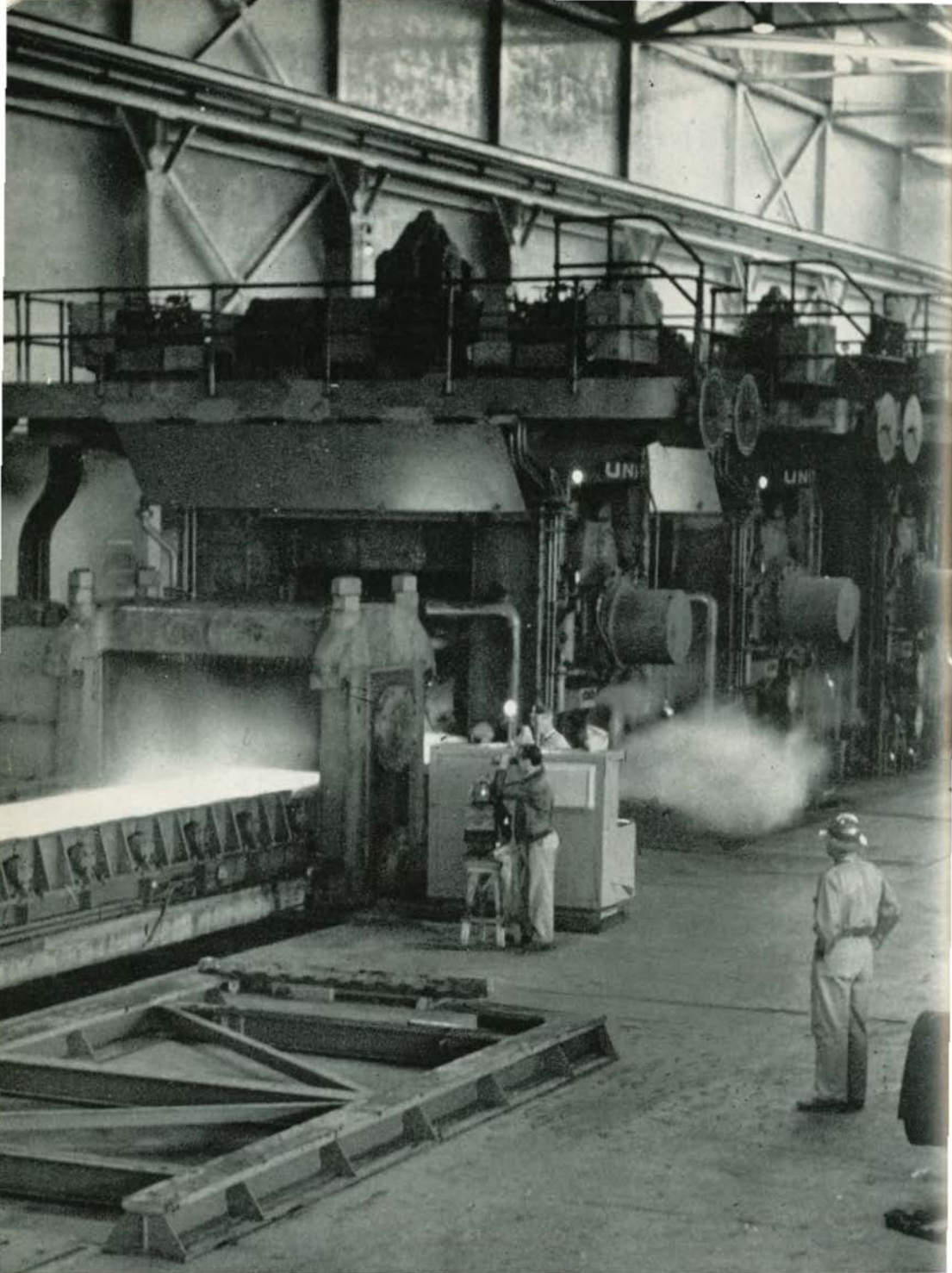
Kaiser Steel's hot strip mill produces hot rolled sheets in coils or cut lengths, in widths from 24 to 72 inches.
