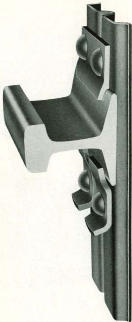
GENERAL ARRANGEMENT M 19 A WITH No. 26 AA-3 CLIP AND TWO No. 26 K CLIPS AFTER ATTACHING THE RAIL
