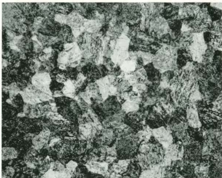
Grain size by etching of fully hardened martensite Fig. 35, Above. Grain size No. 2 Fig. 36, Below. Grain size No. 4
