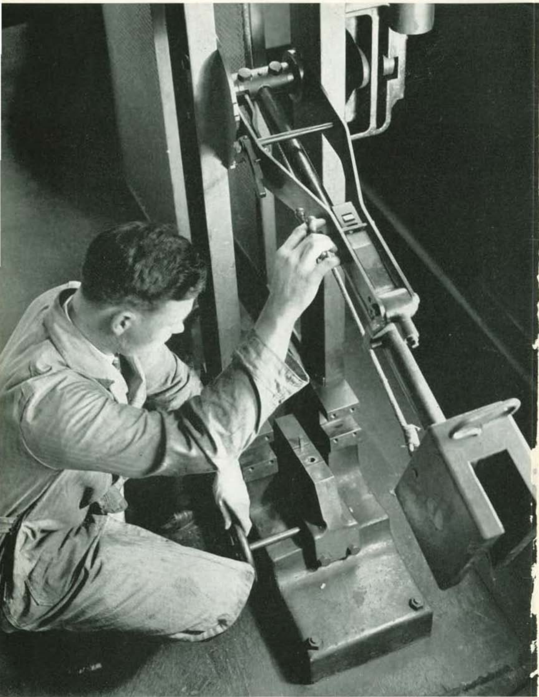
Testing the toughness of steel by breaking it in an impact testing machine
