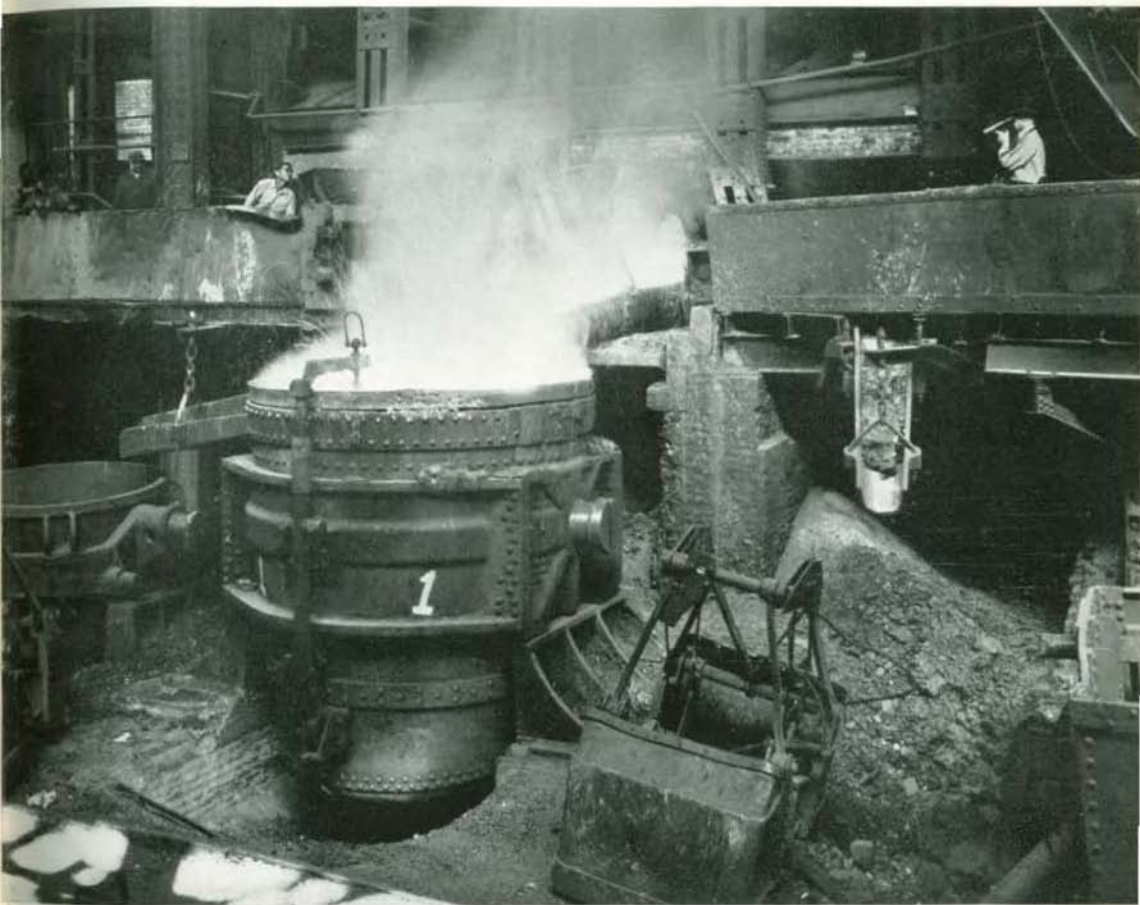
Tapping an open hearth. As the molten metal flows into the ladle in the foreground, the observer at the right is taking its temperature with an optical pyrometer
