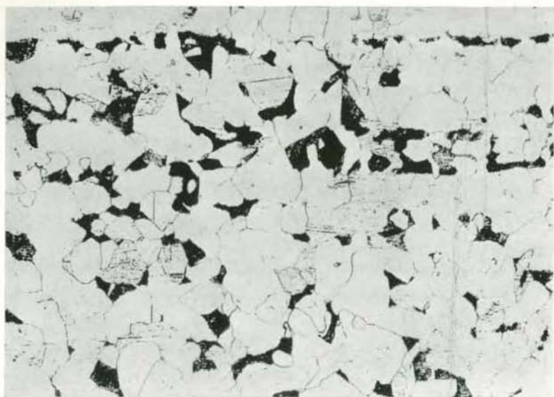
Fig. 29. Grain size test showing structure before heating
