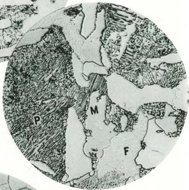
Fig. 3. 0.43% carbon steel quenched from 1320°F. M—martensite
