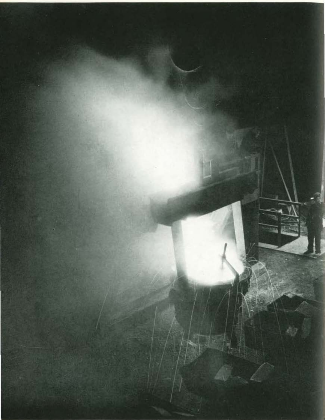
At the right a workman is checking the temperature with an optical pyrometer as this heat is tapped
