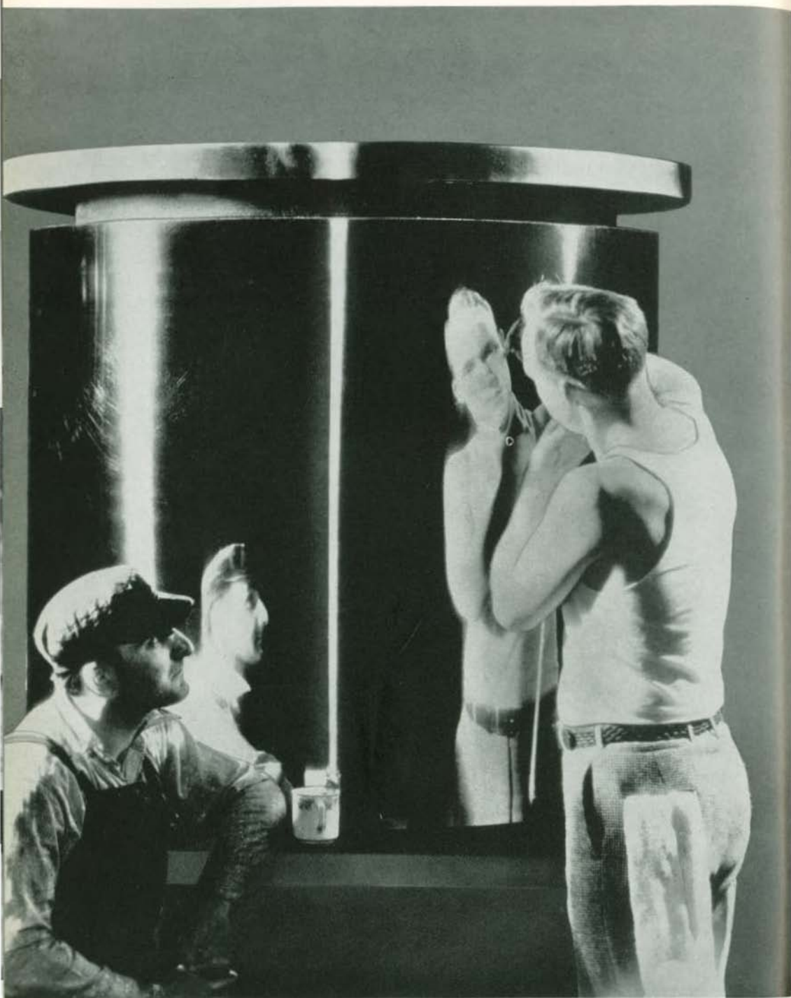
The perfect mirror finish of this giant rollneck bearing made of U-S-S Carillo Alloy Steel is remarkable because it is merely ground, not polished
