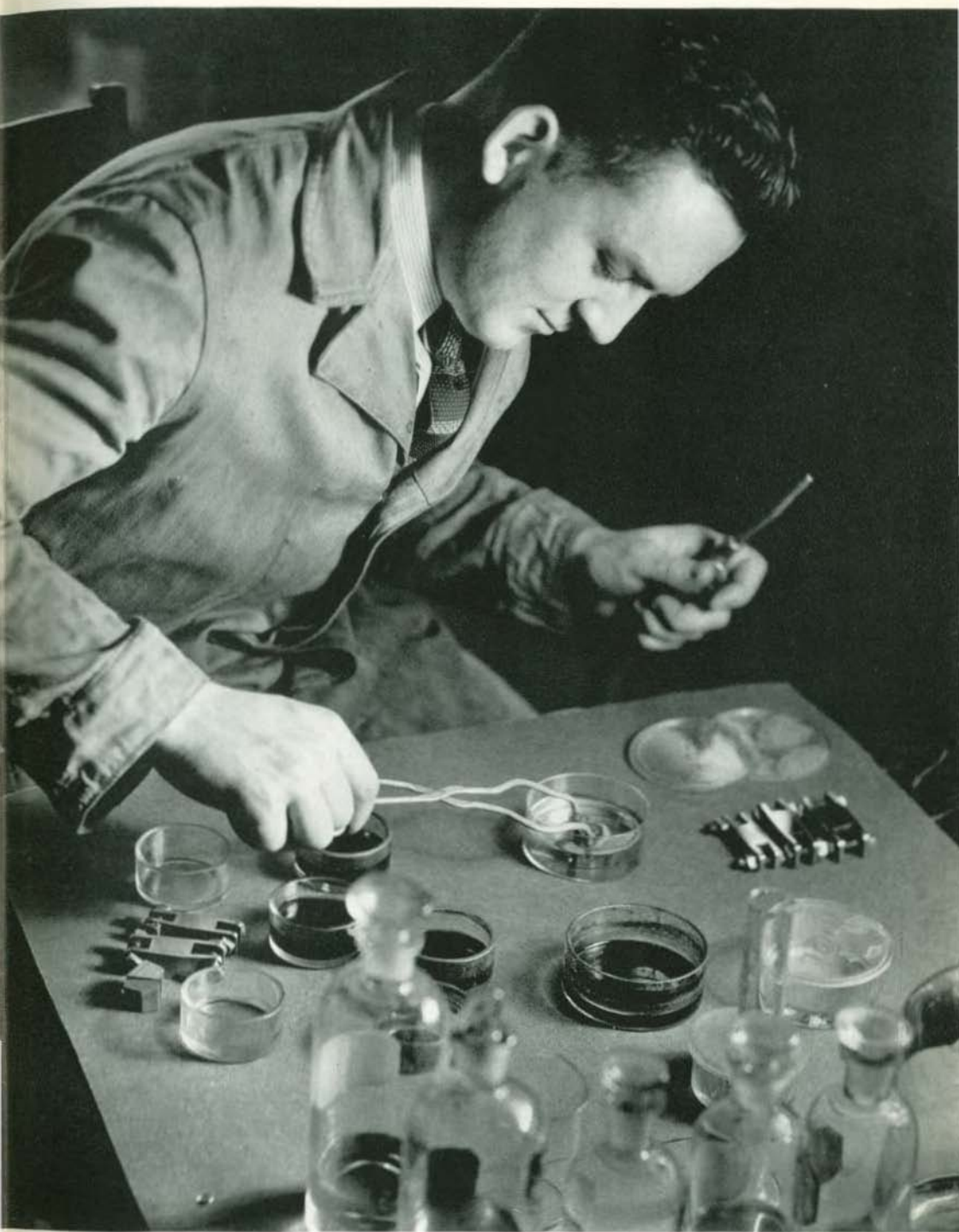
Etching a specimen of steel for subsequent examination under the microscope
