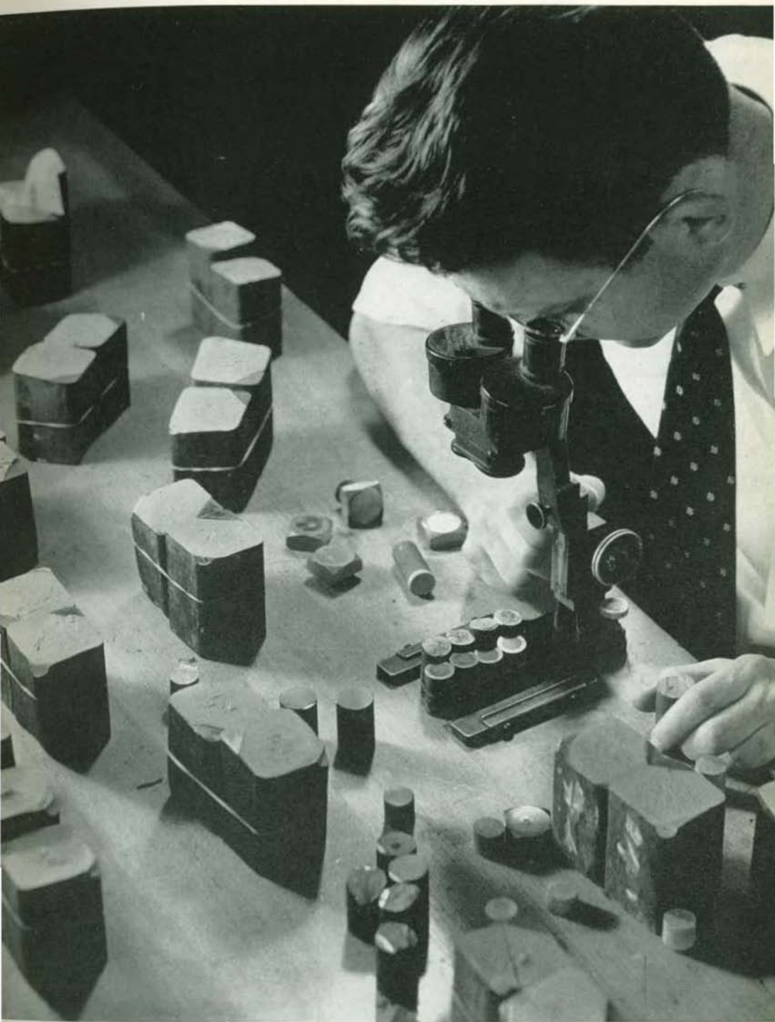
Ascertaining hardenability by examining fractured pieces and etched sections
