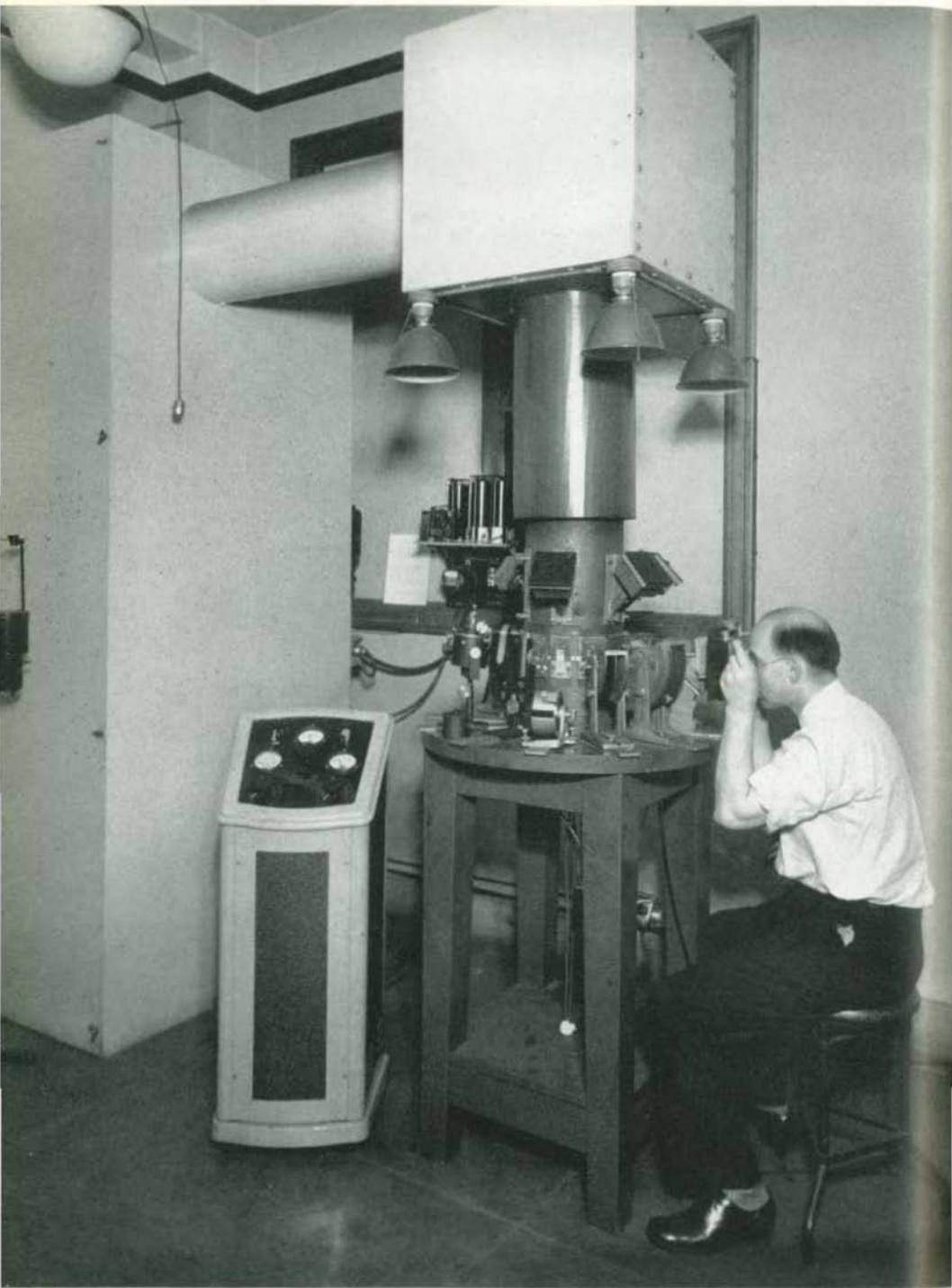
Setting up X-ray equipment for ascertaining the crystal structure of metal
