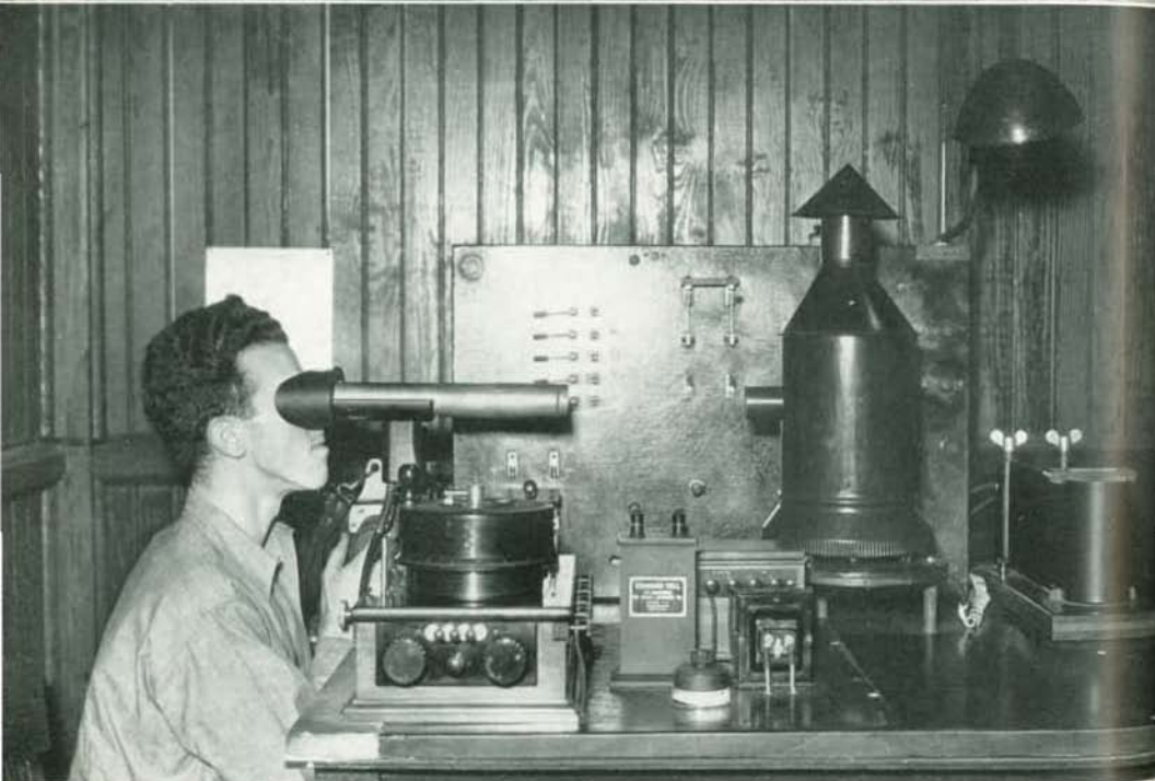
Above: Rolling experimental pieces in the 6-inch experimental rolling mill Below: Calibration of optical pyrometers to be used in the measuring of temperature of liquid steel from furnaces or solid steel in rolling mills
