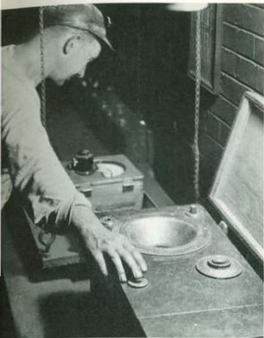
An open hearth melter making a rapid and accurate determination of the carbon content of the steel he is melting
