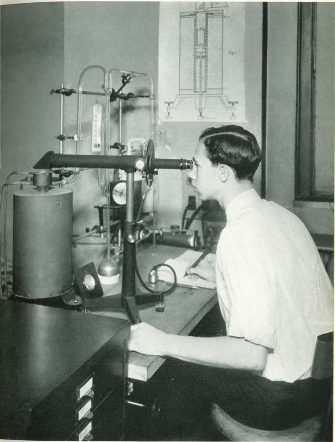
Determining the thermal expansion of metals and refractories in vacuum, air or other gases
