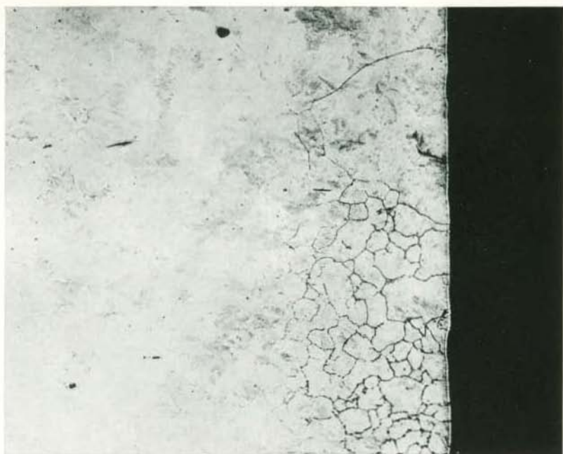
Fig. 31. Structure of the steel of Figs. 29 and 30 after carburizing for 8 hours at 1675° F. Sodium picrate etch. X100
