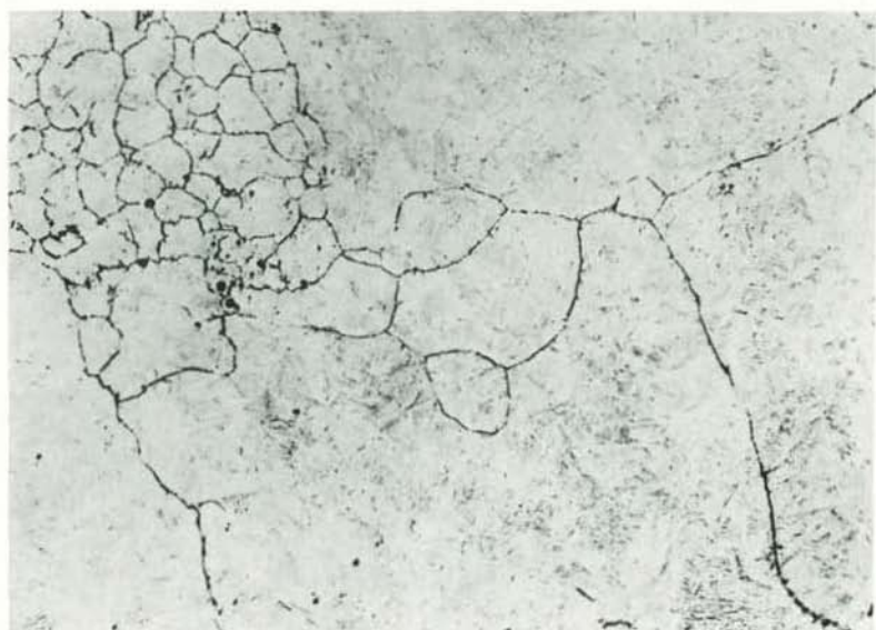
Fig. 32. Structure of the steel of Figs. 29, 30, and 31 after carburizing for 8 hours at 1700° F. Sodium picrate etch. X100
