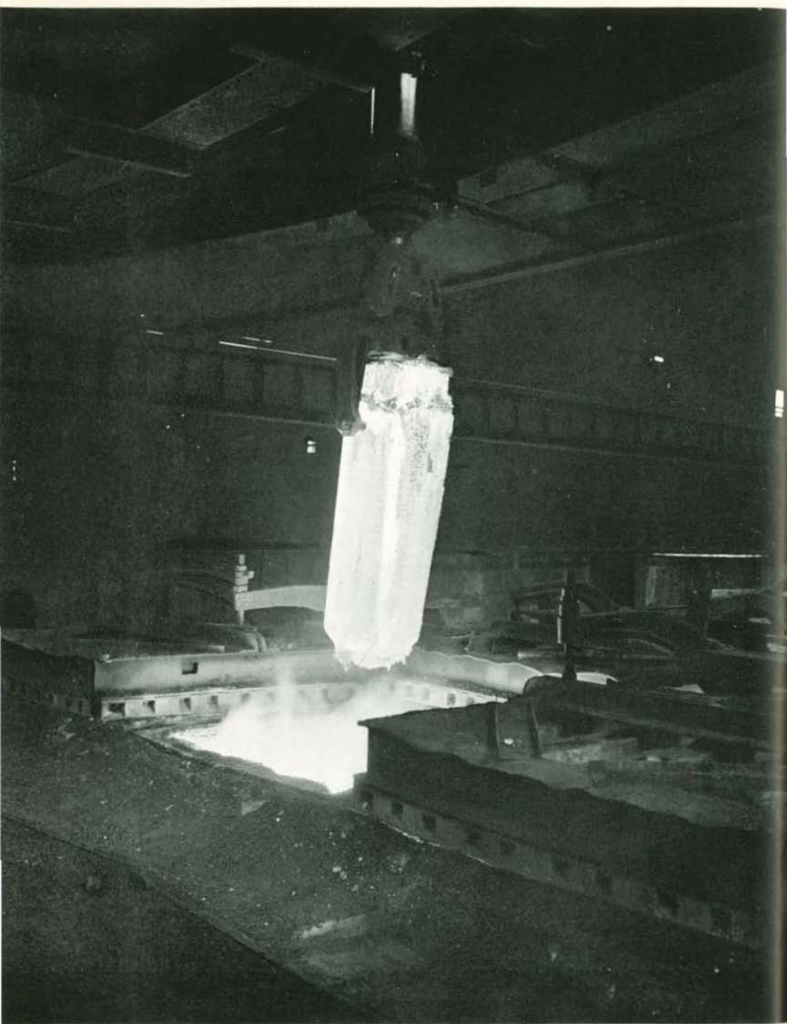
Ingot of steel being lifted from soaking pit after it has been heated to the temperature necessary for subsequent rolling operations
