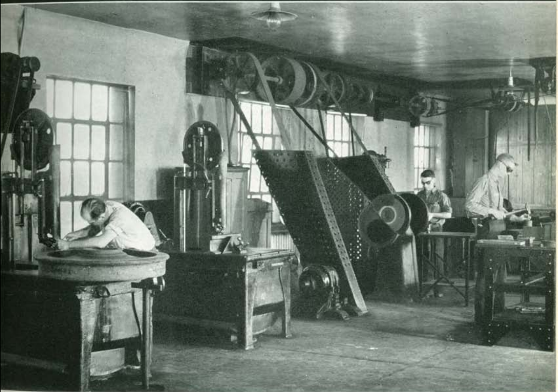
Above: Fatigue machine for testing the behavior of steel under repeated alternating stress Below: Band saws and other laboratory equipment for the preparation of test pieces
