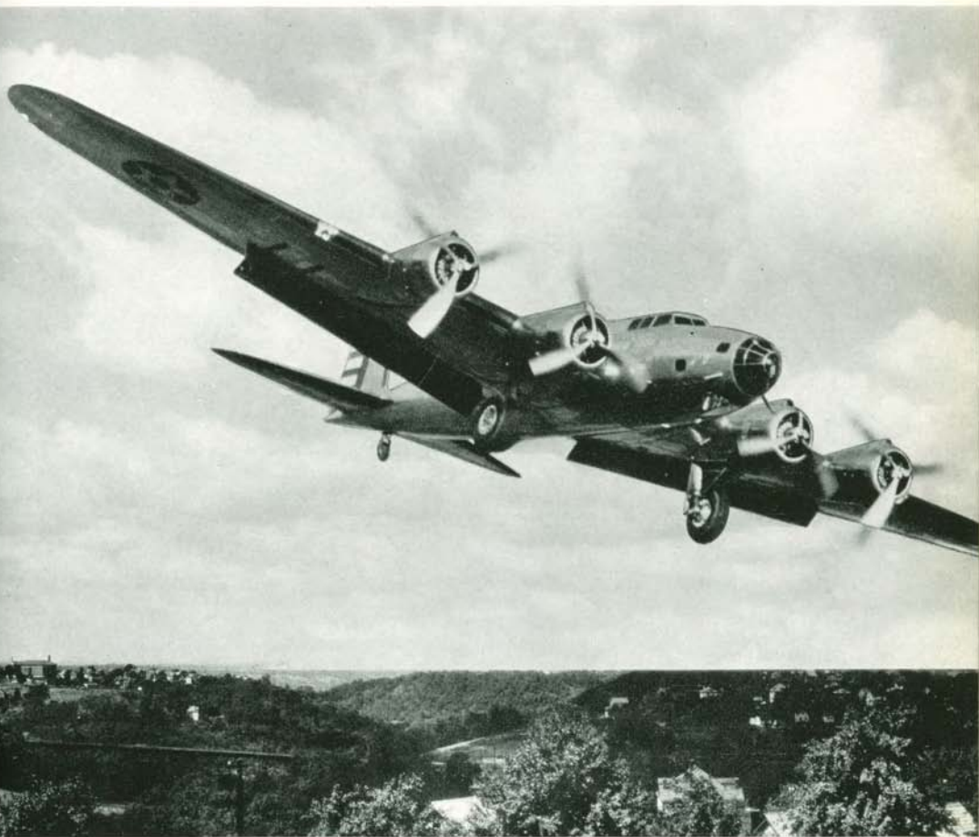
In building this flying fortress, alloy steels such as S.A.E. X-4130 play an important part
