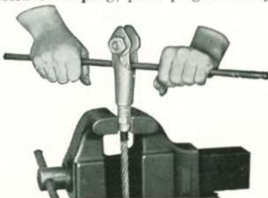
E Socket being screwed down.
