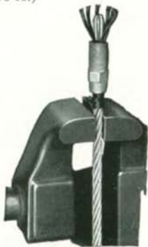
C Strand ends projecting correct distance through sleeve.
