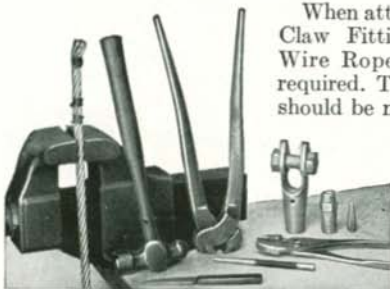
A End of wire rope with one seizing near end and two seizings beyond, also tools to be used.
