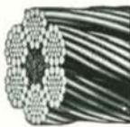
Type G—6 Strands—30 Wires to the Strand—1 Hemp Core
