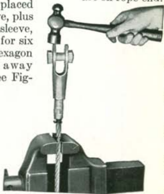
B Sleeve being driven down correct distance.
