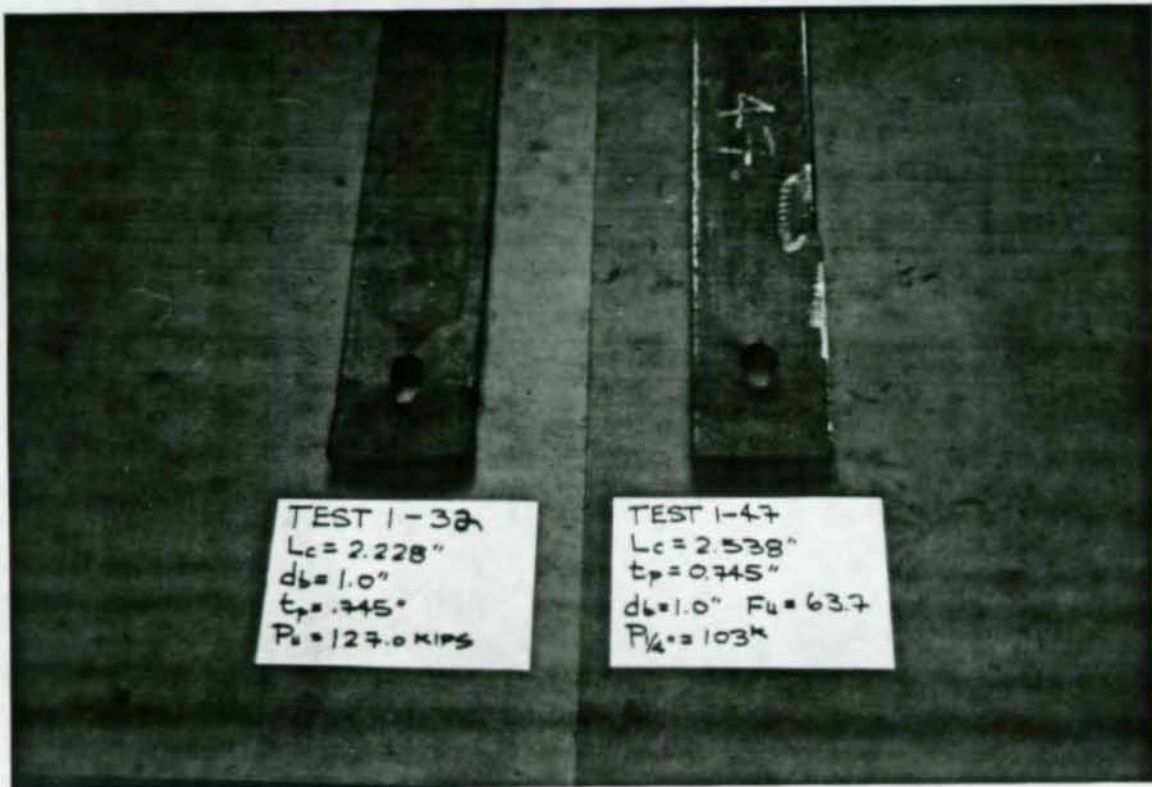
Figure 17. Two Failures for 1 in. Diameter Single-Bolt Specimens with Large End Distances. The specimen on the left was loaded through a large deformation, while the one on the right was stopped at 1/4 in. deformation. The maximum load for the specimen on the left is twenty-three percent higher than for the specimen on the right. There was a bolt failure during the test on the left; therefore, the result is not plotted.
