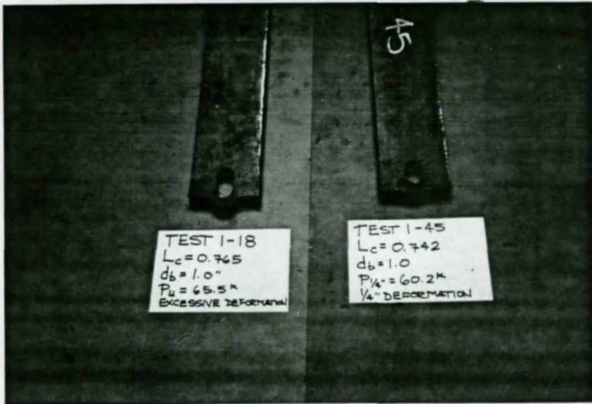
Figure 16. Two Failures for 1 in. Diameter Single-Bolt Specimens with Medium End Distances. The specimen on the left was tested to end tearout, while the specimen on the right was tested to 1/4 in. deformation. The maximum load for the specimen on the left was nine percent higher than for the specimen on the right.
