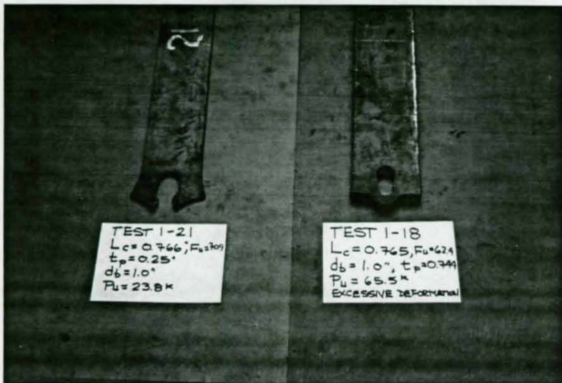
Figure 12. Specimens of Different Thickness with the Same End Distance. For the specimen on the left, t_p = 0.25 in. and F_v/F_u = 1.34 ; for the specimen on the right, t_p = 0.744 in. and F_v/F_u = 1.41 .
