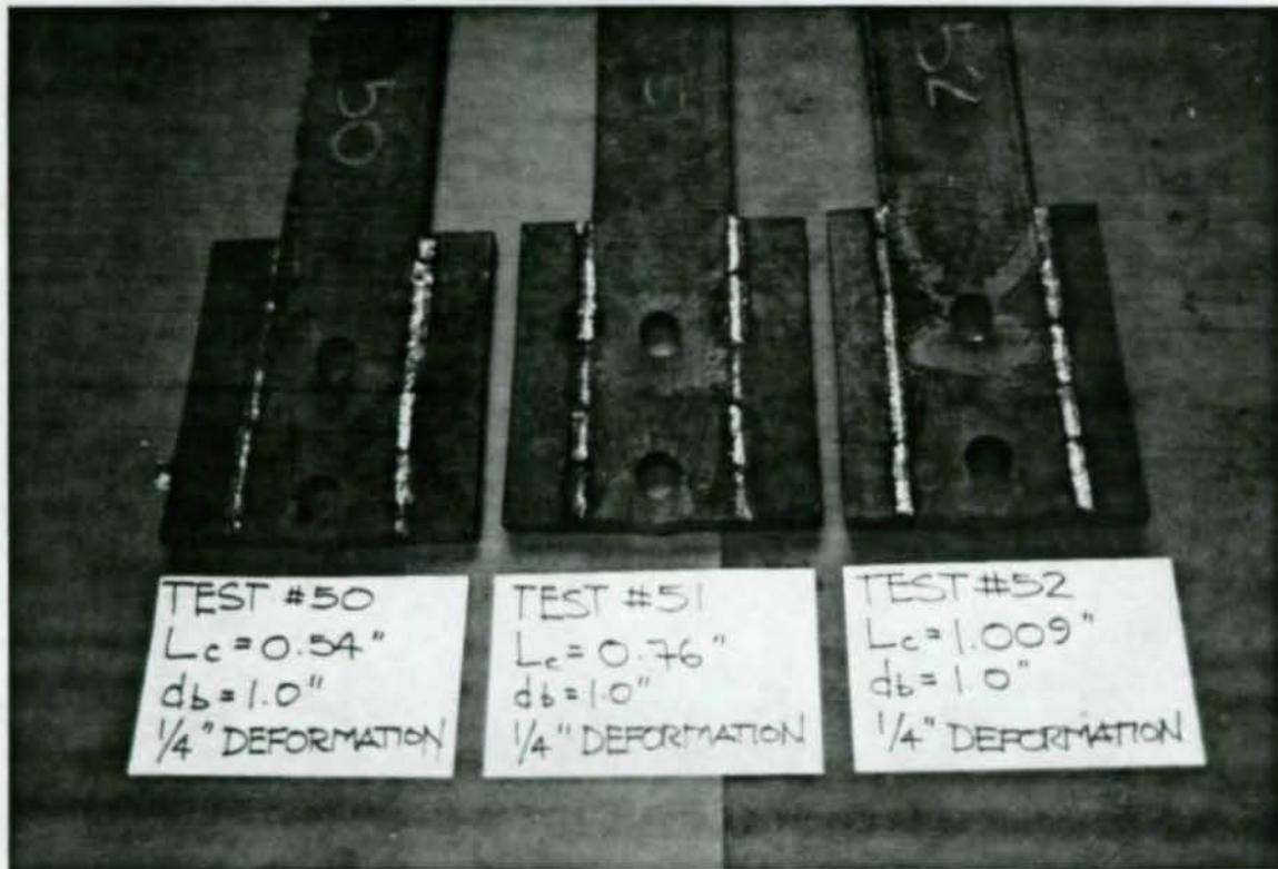
Figure 18. Comparison of 1/4 in. Deformations on Two-Bolt Specimens with 1 in. Diameter Bolts. The failure load for the specimen in the middle is 151 kips. This is less than the additive results from the specimens in Figures 16 and 17 (60.2 kips + 103 kips = 163.2 kips). The clear end distances for the specimens in Figures 16 and 17 are approximately equal to the clear end distance and clear spacing for the specimen in this figure.
