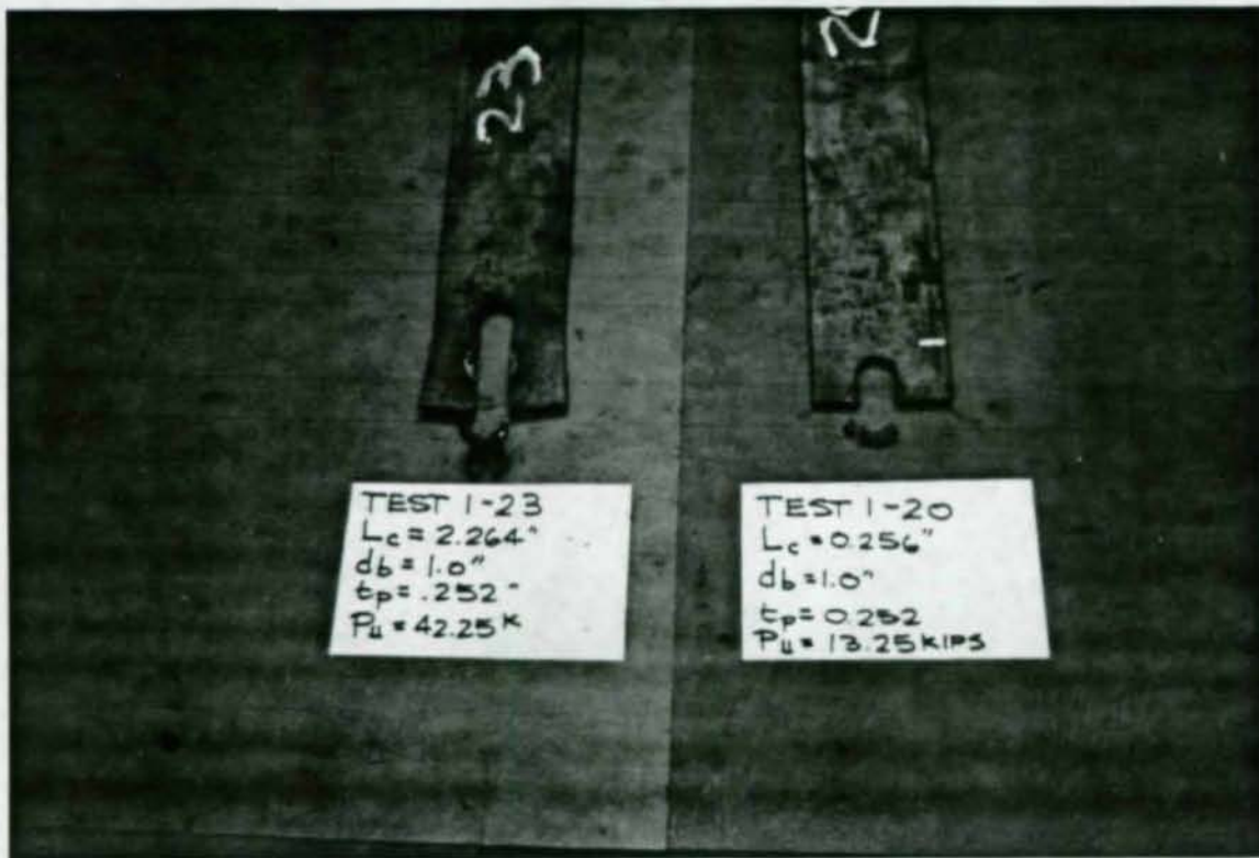
Figure 13. Comparison of End Tear-Out Failures. The specimen on the left with the large end distance experienced a large build-up of material ahead of the bolt prior to tearout. The specimen on the right with the small end distance failed before any large deformations occurred.
