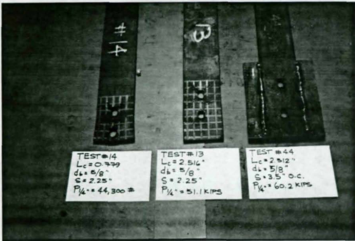
Figure 24. Specimens Built with 5/8 in. Diameter Bolts and Capable of Resisting a Bearing Stress of 2.4F_u According to the AISC/LRFD. Only the specimen with 3.5 in. spacing and 2.512 in. clear end distance is capable of resisting 2.4F_u .
