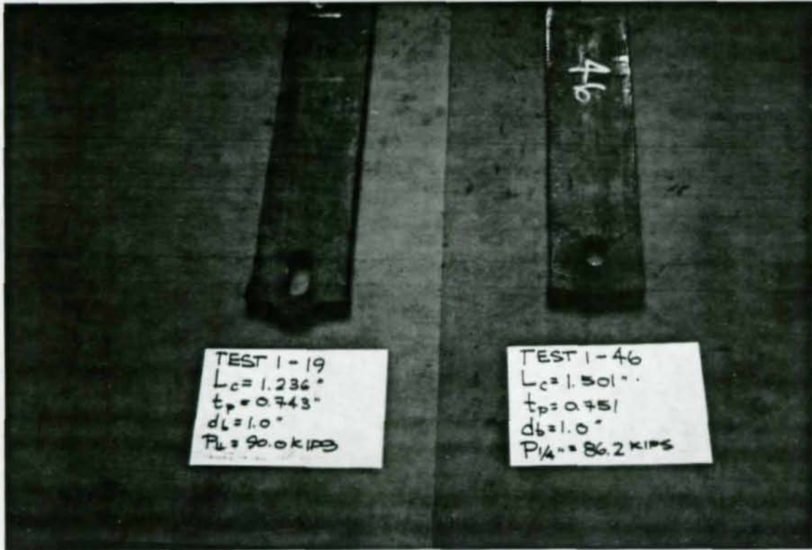
Figure 11. Comparison of Excessive Deformation and 1/4 in. Deformation. The two specimens are of approximately the same configuration. The one on the left was allowed to undergo excessive deformation while the one on the right was stopped at 1/4 in. deformation in the bolt hole.
