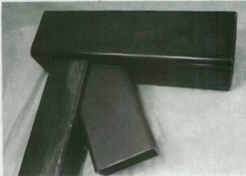
Figure 5. Gapped versus overlapped stepped-box connections. This can also occur with matched-box connections.
