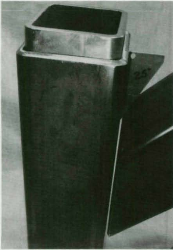
CJP (Key 13). TS 4x4x \frac{1}{4} " with backing ring for future butt splice. TS 4x4x \frac{1}{4} " branch member @ 45° intersection angle. Required bevel in heel zone is 22 \frac{1}{2} 0 min.
