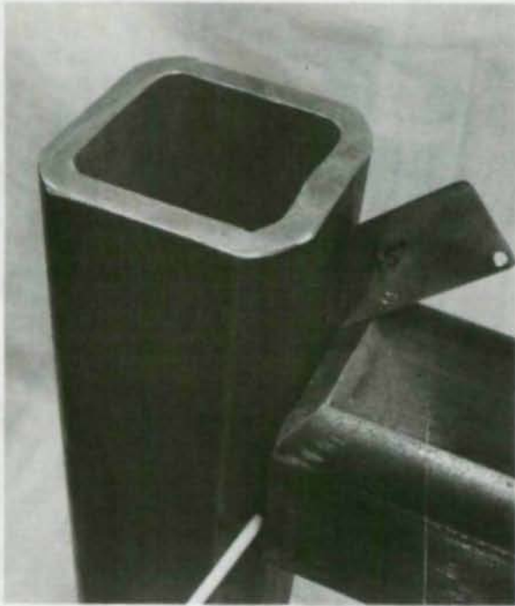
CJP (Key 4). TS 4x4x \frac{1}{2} " with 1/8" electrode.
