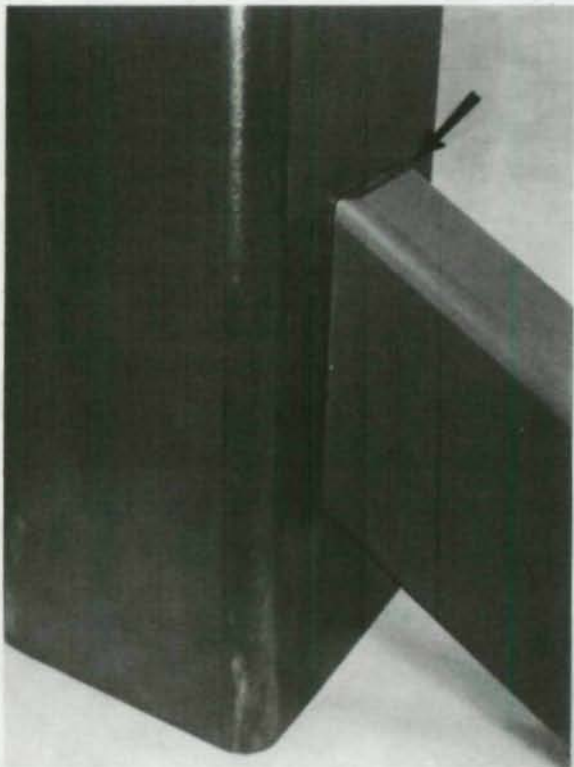
Fillet (Key 21). Note bevel in toe zone only.
