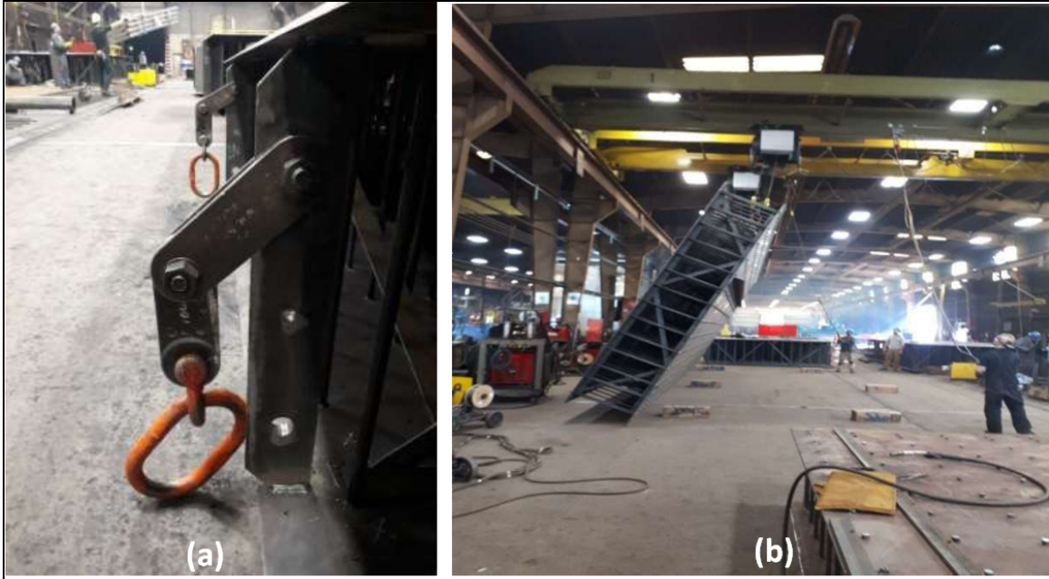
Figure 26: (a) Lifting Attachment on Rainier Square Panel and (b) Rotating a Panel Using the Attachment in the Shop
