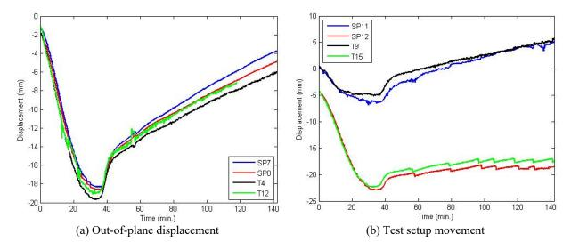
Fig. 2-27. Comparison of measured displacement by string potentiometer and OptiTrack.
