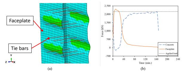
Fig. 3-9. (a) Local buckling of faceplate between tie bars of CW-300-20-20P (b) Force distribution in CW-300-20-20FP between the faceplate and concrete core
