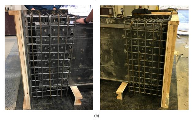
Fig. 2-2. (a) Specimen with welded headed shear studs (b) Concrete blocks steelwork
