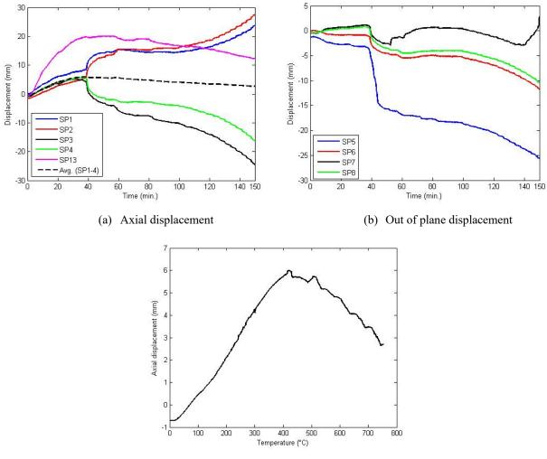
(c) Axial displacement against surface temperature
