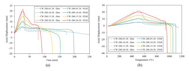
Fig. 4-27. Comparison of fiber-model and FE analysis predicted axial displacements for CW-200 specimens using section method; (a) axial displacement vs time and (b) axial displacement vs surface temperature
