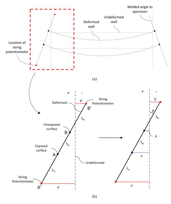
Fig. B1. Schematic plan view of deformed shape of CW2 specimen with the detail
