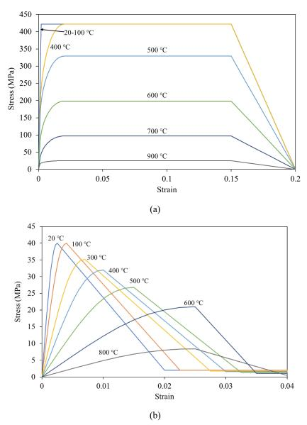
Fig. 4-8. Eurocode stress-strain-temperature curves for (a) 420 MPa steel and (b) 40 MPa concrete
