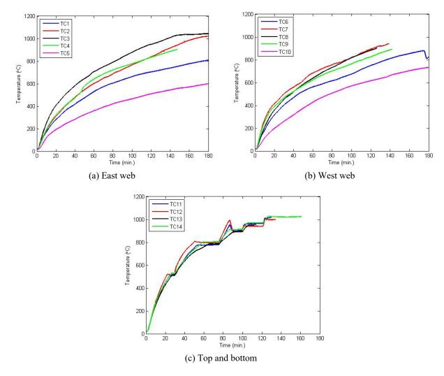
Fig. 2-16. The surface temperature of CW1 (Test 2)
