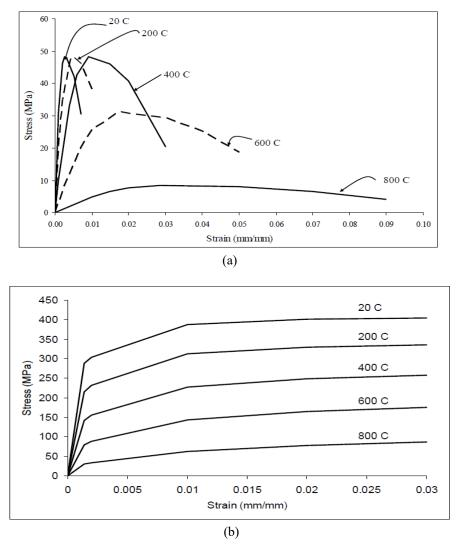
Fig. 4-7. Concrete (a) and steel (b) stress-strain curves at elevated temperatures developed by Lie. (Hong, 2007)
