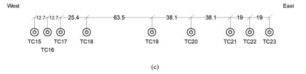
Fig. 2-10. (a) The layout of thermocouples installed on the West web (East) (b) the thermocouples installed on the Top flange (Bottom) (c) Layout of thermocouples placed within the thickness of the specimen (Dimensions are in mm).
