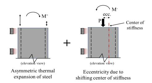
Fig. 4-36. Representation of the two types of moments generated in a wall section exposed to asymmetric heating
