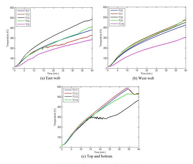
Fig. 2-13. The surface temperature of CW1 (Test 1)
