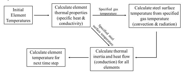
Fig. 4-3. Schematic flowchart of algorithm for 2D heat transfer
