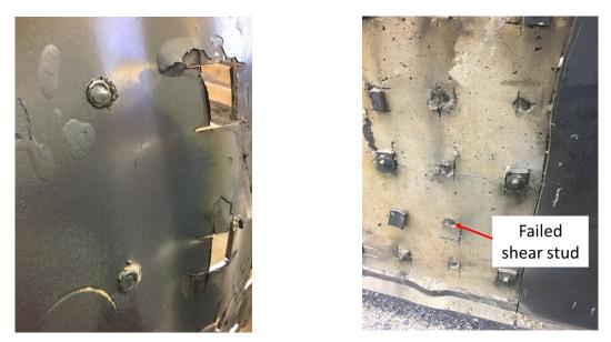
Fig. 2-19. Failed shear studs after the fire test
