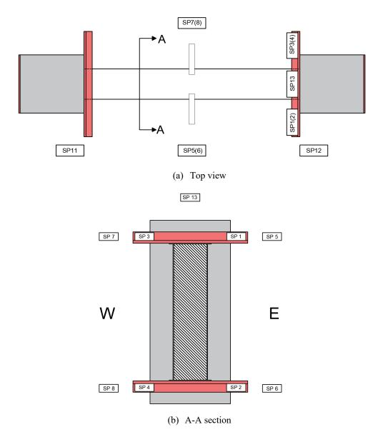
Fig. 2-11. The layout of the string potentiometers
