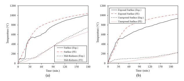
Fig. 3-4. Comparison of predicted temperatures from the FE analysis with the experimental (Exp.) data at different sections for SCW7 (a), SCW12 (b)
