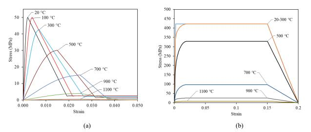
Fig. 3-2. Stress-strain relation of concrete (a) and steel (b) at elevated temperatures per Eurocode 3
