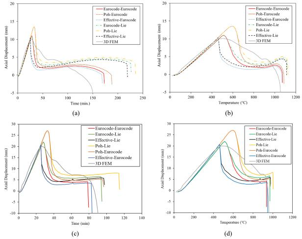
Fig. 4-14. (a,c) Axial displacement vs time and (b,d) Axial displacement against temperature for the wall specimen for different combinations of material models, plotted with the FE analysis obtained curve. The curves are labelled by the steel and concrete model, respectively.
