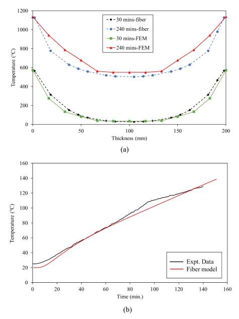
Fig. 4-13. (a) Temperature profiles across the section at various time instants; Comparison of fiber model predicted and FEM data. (b) Surface temperature vs time for 3-sided heating: comparison of experimental data and fiber model. The plot shows the temperature of a point on the un-heated surface
