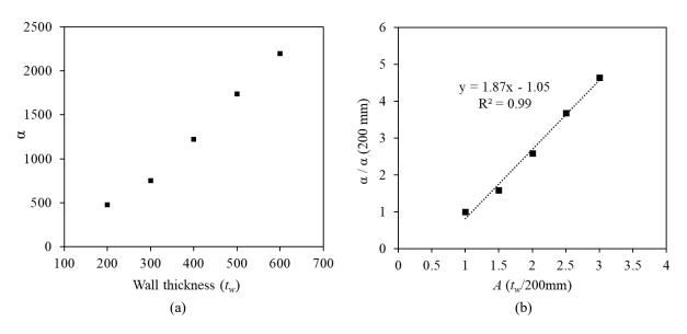
Fig. 3-22. The relation of the wall thickness and the constant ( $\alpha$ ) in Eq. (3-15)
