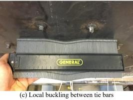
Fig. 2-36. Local buckling in the specimen between tie bars after the fire test CW4 (Test1)
