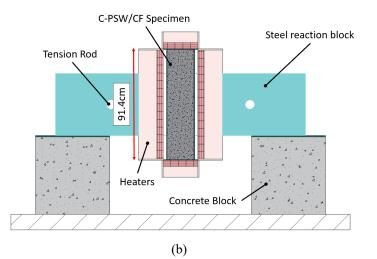
Fig. 2-7. (a) Arrangement of heaters (b) Placement of specimen and heaters in the test setup
