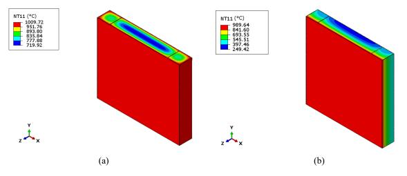
Fig. 3-3. Temperature distribution for (a) Uniform fire and (b) One-sided fire conditions after 3 hours of fire exposure
