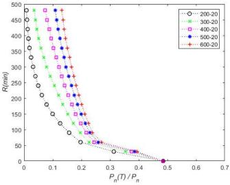
Fig. 3-20. Calculated fire resistance rating versus applied load ratios for C-PSW/CFs with various wall thicknesses and wall slenderness ratio of 20
