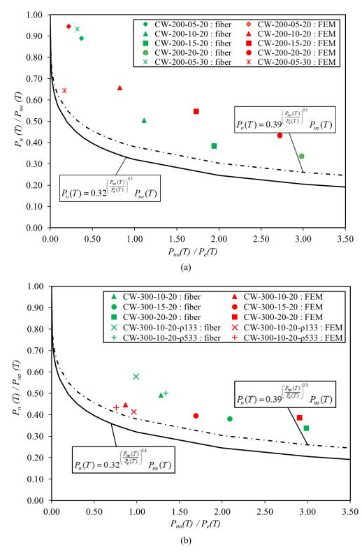
Fig. 4-26. Normalized results of the comparison between fiber-model and FE analysis for wall specimens using section method for (a) 200 mm wall thickness and (b) 300 mm wall thickness
