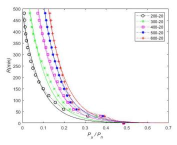
Fig. 3-21. Fitted curves for calculated fire ratings of C-PSW/CFs against applied load ratio.
