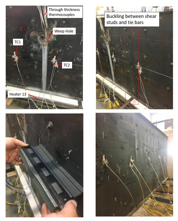
Fig. 2-15. Local buckling in CW1 specimen after the fire test
