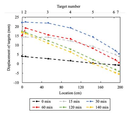
Fig. 2-28. Movement of the specimen within the test setup at different time points
