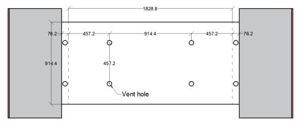
Fig. 2-37. Location of vent holes in CW4 (Test2). Dimensions are in mm.
