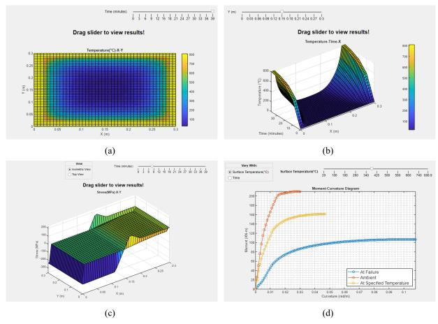
Fig. 4-17. Examples of post-processor output interfaces
