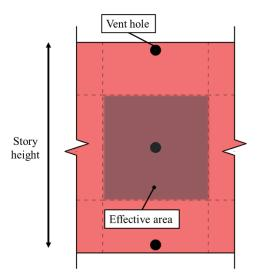
Fig. 5-2. Vent holes located at the center of effective area, bottom and top of walls at every floor
