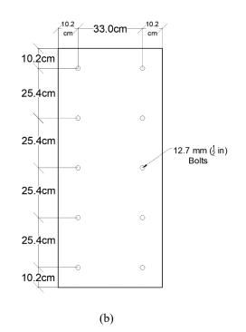
Fig. 2-1. (a) Foundation block design detail (b)The location of holes in the backplate
