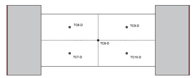
Fig. 2-20. The layout of thermocouples on the unexposed surface of the specimen
