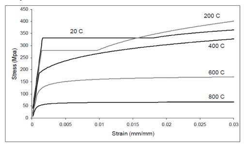
Fig. 4-6. Stress-strain curves for 330 MPa steel developed using Poh's model. Ref: Hong (2007)
