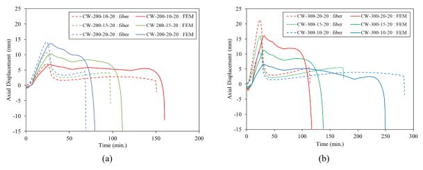
Fig. 4-30. Comparison of fiber-model and FE analysis predicted axial displacements for (a) CW-200 specimens and (b) CW-300 specimens using strip method
