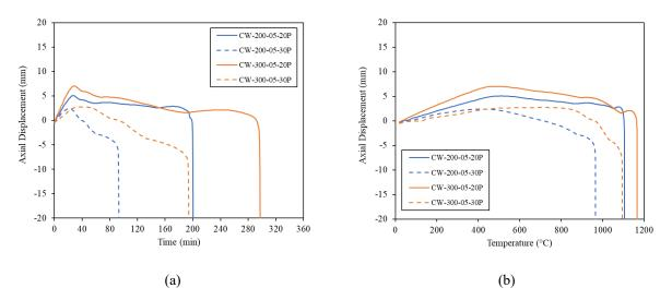
Fig. 3-12. Axial displacement of walls under three various load ratios CW-200s against time (a) and wall surface temperature (b)
