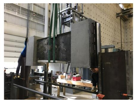
Fig. 2-5. Placing CW1 in the test setup
