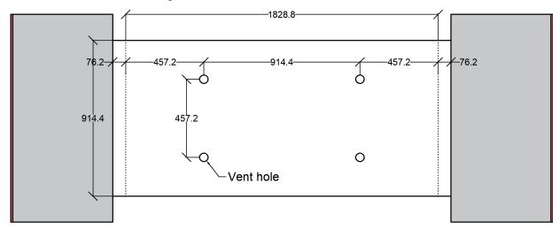
Fig. 2-30. Location of designed vent holes on CW3. All dimensions are in mm.
