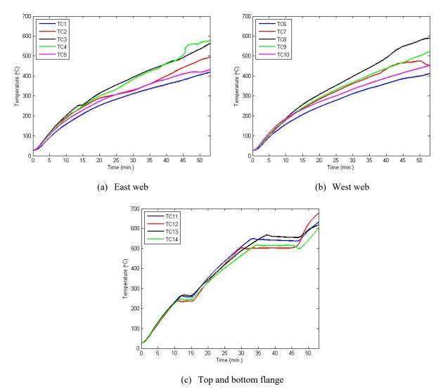
Fig. 2-34. The measured surface temperature of CW4 (Test1)
