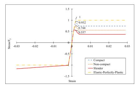
Fig. 4-9. Effective stress-strain curves for compact ( $\lambda$ =50), non-compact ( $\lambda$ =67) and slender ( $\lambda$ =100) sections for steel (F<sub>y</sub>=358 MPa) at ambient temperature
