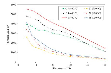
Fig. 4-21. Critical load versus slenderness curves at two surface temperatures for varying concrete compressive strength
