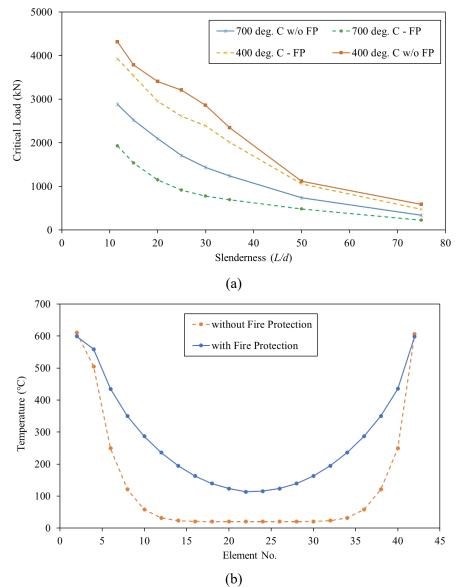
Fig. 4-22. (a) Critical load vs Slenderness comparison for a column with and without fire protection. (b) Temperature profiles for a column at failure with and without FRP for steel surface temperature =  $600 \text{ }^{\circ}\text{C}$
