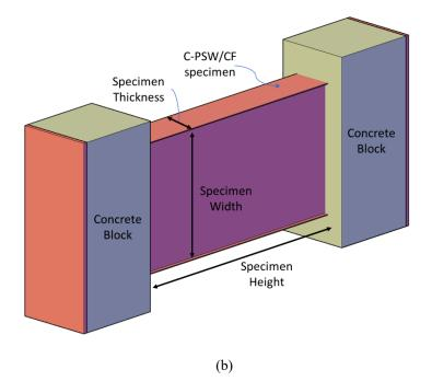
Fig. 2-3. (a)Specimen with concrete blocks after pouring concrete (b) schematic drawing of the specimens
