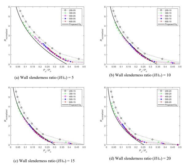
Fig. 3-23. The fitted curve for various wall slenderness ratios (Power format)
