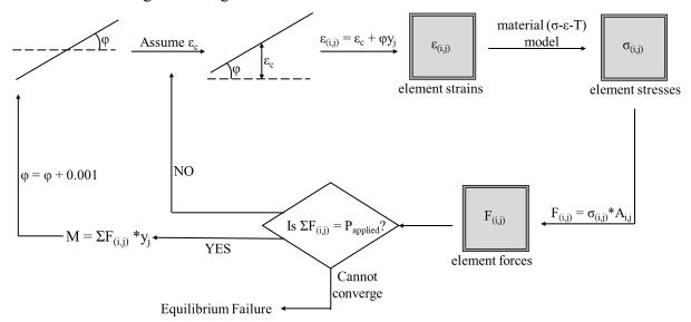
Fig. 4-4. Pictorial flowchart for calculating section moment-curvature response
