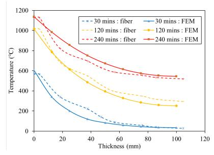
Fig. 4-28. Temperature profiles comparison (half-section) between fiber-model and FE analysis for 200mm wall thickness at three time instants- strip method
