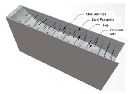
Fig. 1-1. Details of a Composite Plate Shear Wall/Concrete Filled (C-PSW/CF)
