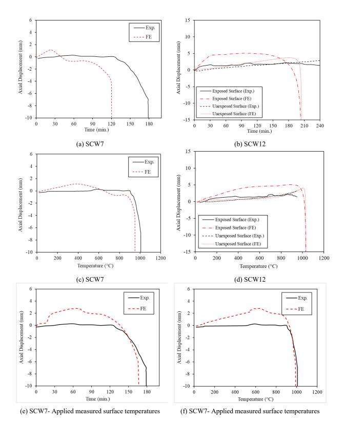
Fig. 3-5. Comparison of axial displacement against time or surface temperature for SCW7 and SCW12
