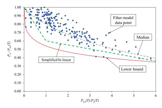
Fig. 4-25. Normalized results of the parametric studies plotted with the proposed theoretical capacity curves (lower-bound, median and simplified bi-linear)
