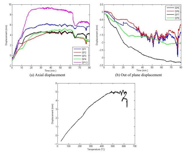
(c) Surface temperature against axial displacement
