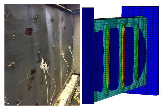
Fig. 3-7. Local buckling of faceplate in CW3
