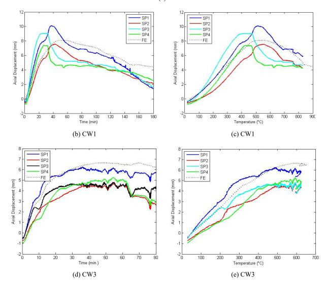
Fig. 3-6. Comparison of axial displacement against time for CW1 and CW3
