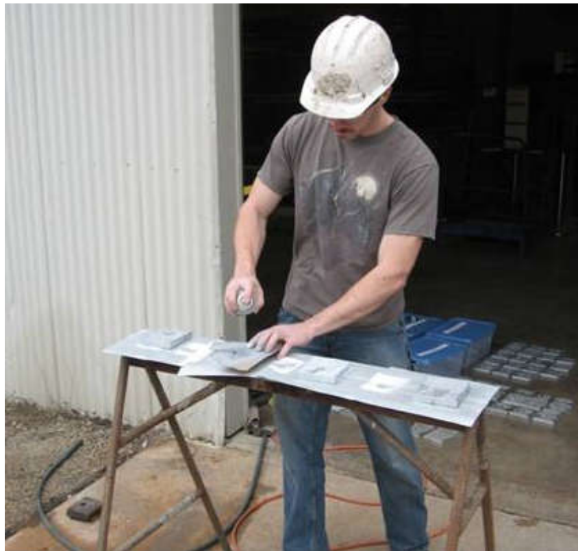
Figure 4 - Spraying Zinc-Rich Paint over Uncoated Areas of Specimens
