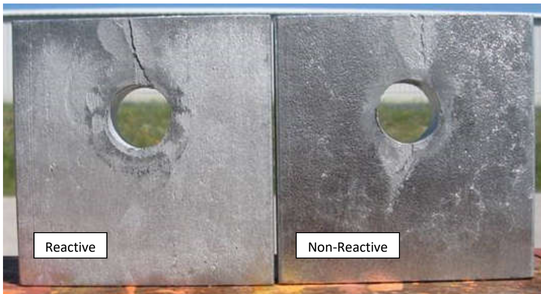
Figure 17 - Different Surface Conditions of Reactive and Non-Reactive Steel
