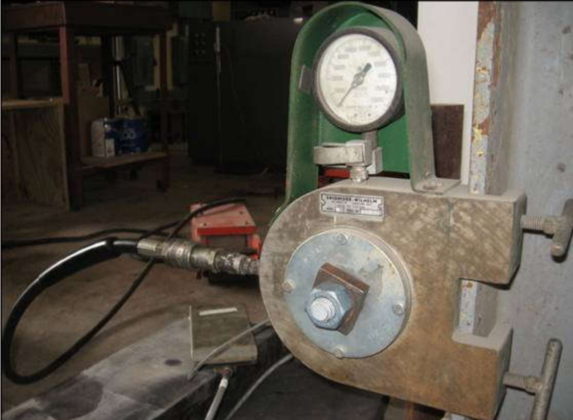
Figure 27 - Calibration of Gaged Bolt through Hydraulic Tension Calibrator
