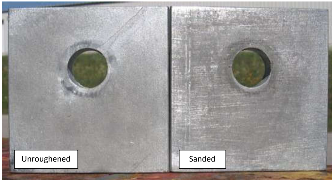
Figure 19 – Un-roughened and Sanded Appearance of High Silicon/Reactive Steel
