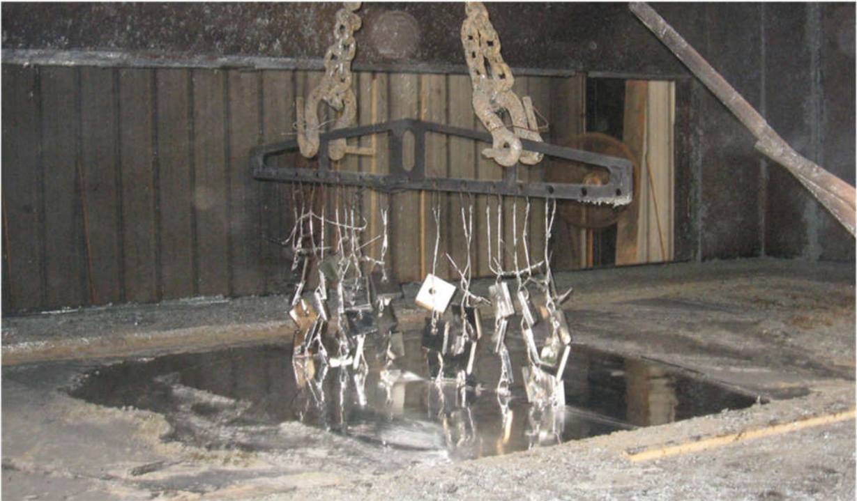
Figure 2 - Dipping Test Plates into Zinc Bath
