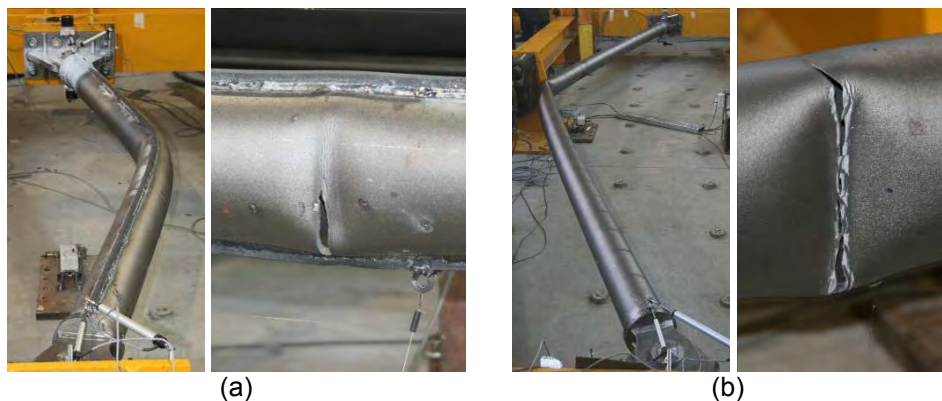
Figure 10. Failure mode of the SP27-2 (a) and SP59-1 (b) specimens.
