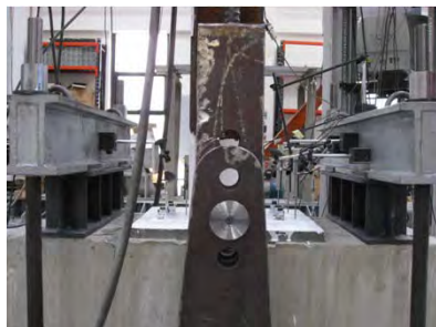
Figure 4. Location of LVDT transducers
