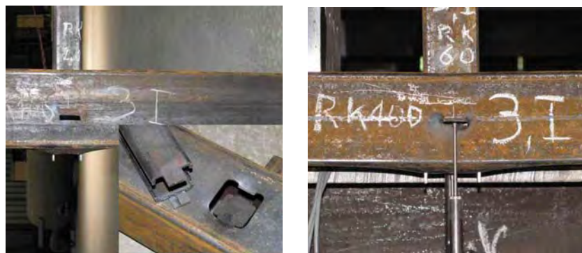
Figure 4. Joint WT2L1 after test (detail of branch in right corner); Joint WT2L2 (bottom wall failure).
