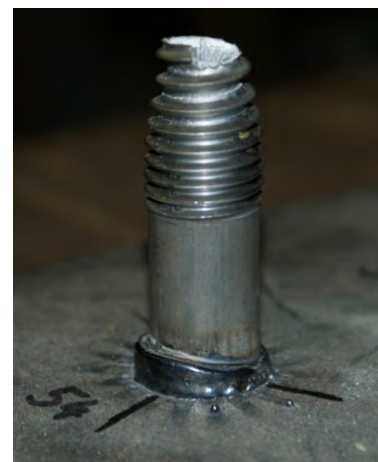
Figure 2.4. Test stud M20x100-PD; failed in threaded part of the stud
