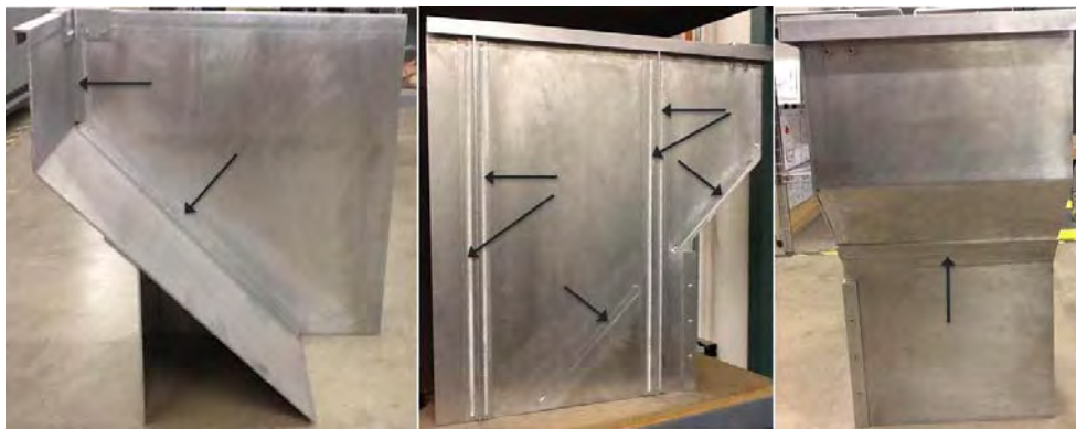
Figure 6. Front, side and rear views of a fabricated shape using multiple orientations of friction stir lap welds (location of welds indicated by arrows).
