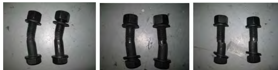
Figure 7. Deformation of the bolts at collapse in tests under axial and shear load.
