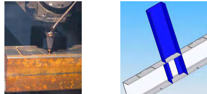
Figure 1. Laser cut of lock & concept of T joint
