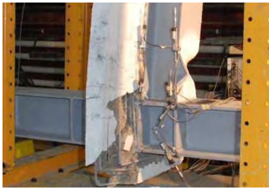
Figure 16. RBS plastic hinges in case of the DB-C_RLD (left) and DB-Comp_RLD (right) specimens.
