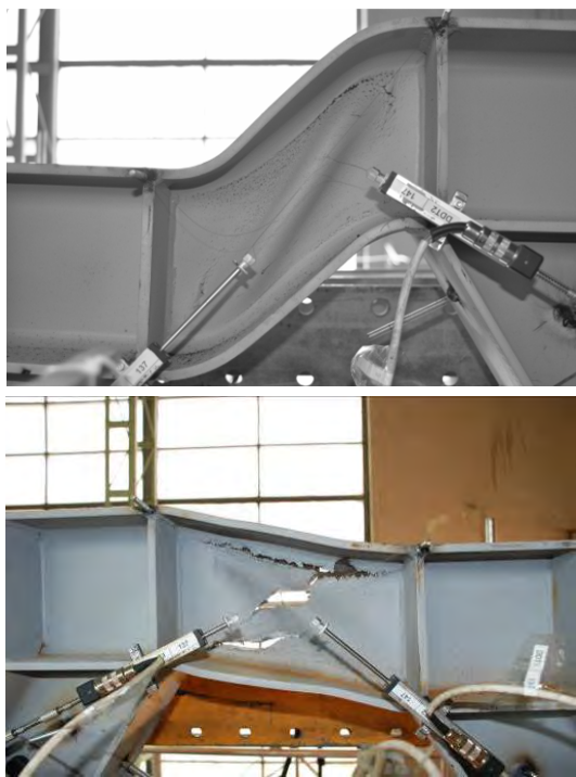
Figure 7. Failure of the link zone for the EBF_M_LF-C (left) and EBF_M_LF-C (right) specimens.
