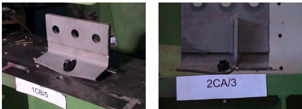
Figure 6. Residual displacements at collapse for tensile tests.
