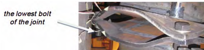
Figure 5. Strongly deformed end plates after test TE1 ( t_{pn}=10 mm).
