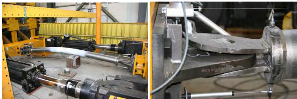
Figure 9. Failure mode of the SP27-1 specimen.
