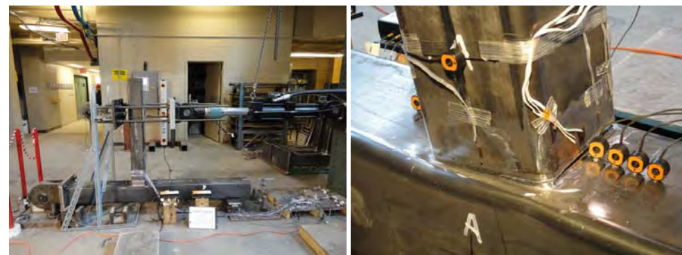
(a) Elevation view of the test setup assembly (b) Shear failure along the weld effective throat
