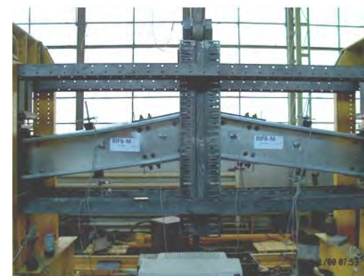
(a) Ridge specimen (RIS-FB-M) experiment
