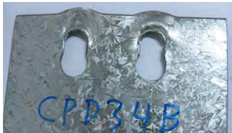
Figure 2. Shear-out of individual bolts
