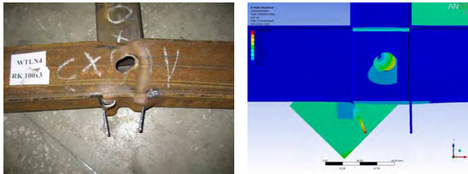
Figure 6. Joint WTLN4 ( \beta = \eta = 0,80 ; \lambda_0 = 33,0 ): after test & numerical model
