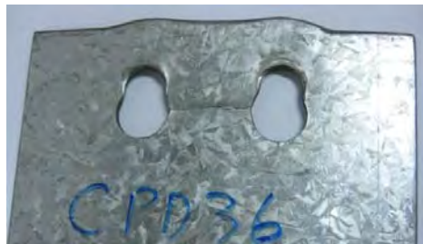
Figure 3. Shear-out deformations gave way to block shear failure
