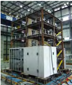
Fig.1 Full-scale building specimen
