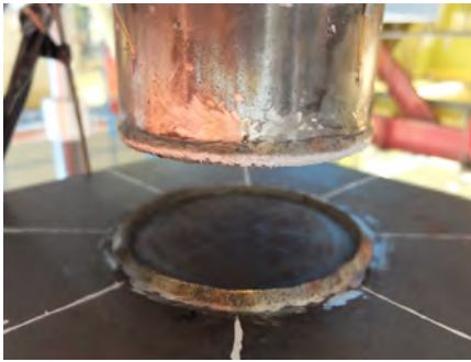
Figure 5. Rupture of connection no. 4
