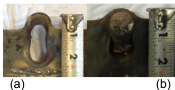
Figure 4 Lap splice joints after testing for plate bearing failure mode (a) Specimen 3-PB-600, Plate 1, (b) Specimen 3-PB-600, Plate 2
