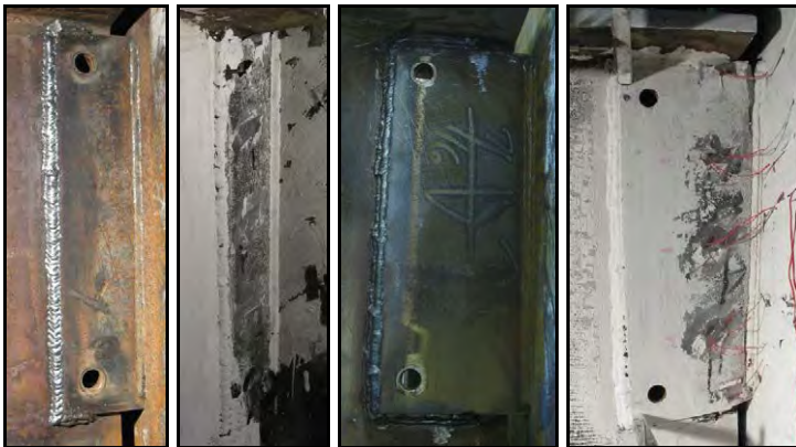
Figure 10: Photographs of post-test deformations for welded connections “Partial C” weld on replacement shear tab plate (Test Configurations 12 & 13)
