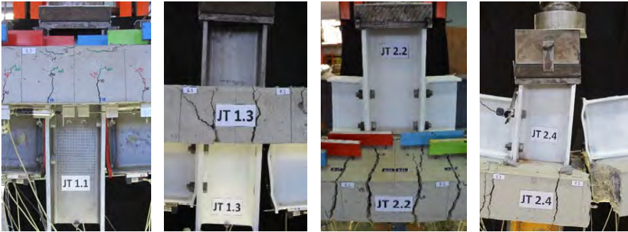
Figure 3. Composite joints after failure (Kuhlmann and Hoffmann, 2015b)
