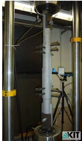
Figure 7. Test adhesive bonded tube specimen setup C (Ummenhofer et al. 2015)
