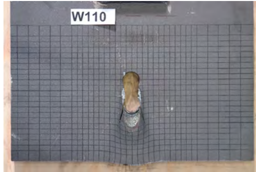
Fig. 5: Failures of W108 ( e_1 = 5db ; e_2 = 3.4db ) and W110 ( e_1 = 5db ; e_2 = 7.5db )
