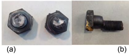
Figure 2 Bolt shear fracture for specimen BS-4 (600°C)
