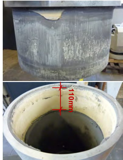
Figure 19: fracture appearance full scale components (Ummenhofer et al. 2015)
