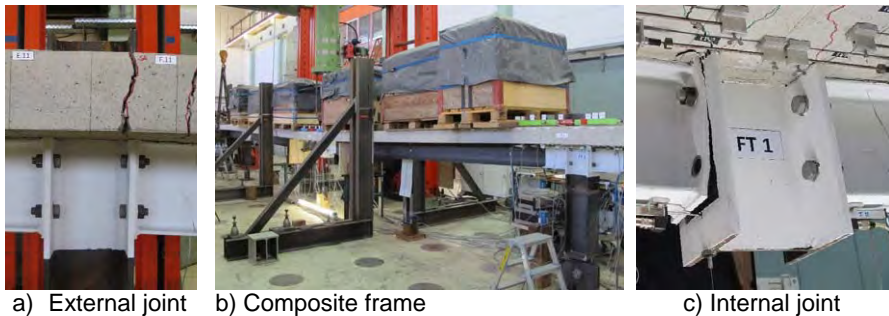
Figure 9. Deformed frame test FT1 at the end of the test
