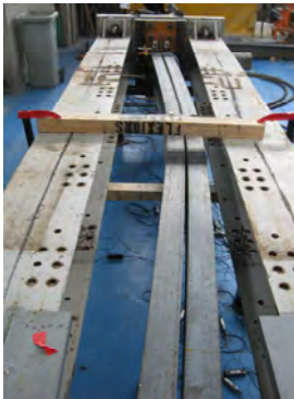
a- Brace global buckling
