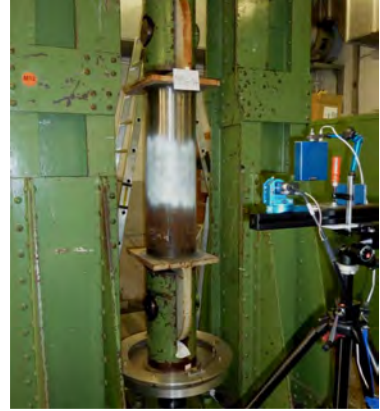
Figure 17: Testing of full scale-component in 3 MN testing machine
