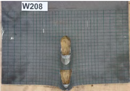
Fig. 6: Failures of W208 ( e_1 = 1.5db ; p_1 = 3.0db ) and W212 ( e_1 = 4db ; p_1 = 3db )
