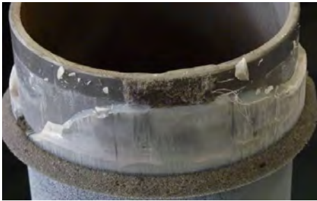
Figure 10a: Fracture appearance inner tube (Ummenhofer et al. 2015)
