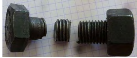
b- Bolt shear failure
