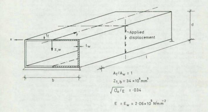
Fig 1 <u>Cross section used for parametric</u> study (webs remain elastic)
