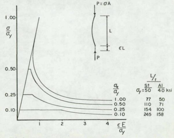
FIG. 2 - MEAN AXIAL STRESS VS EFFECTIVE STRAIN
