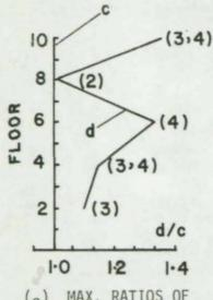
(e) MAX. RATIOS OF AXIAL FORCES, d/c, OF BRACINGS, (), c=N-s, P- $\Delta$ (DL): d-N-S, E-W, P- $\Delta$ (DL) FOR (I)
