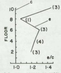
(f) MAX. RATIOS OF AXIAL FORCES, e/c, OF BRACINGS, (), c=N-S,  $P-\Delta(DL)$ ; e=N-S, E-W, VE,  $P-\Delta(DL+VE)$  FOR (I)
