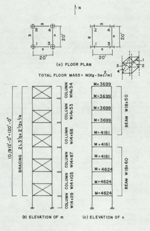
(d) TEN STORY STEEL BUILDING WITH R.C. SLABS AND STEEL BRACINGS FOR (I) DOUBLY SYMM. COLS. AND (II) SINGLY SYMM. COLS. EL CENTRO, 1940, (1 ft = 0.305 m)
