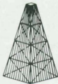
Fig. 5.9 Trussed tubular frame with sloping exterior columns
