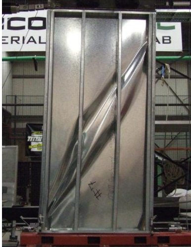
Figure 4: Shear buckling of steel sheet
