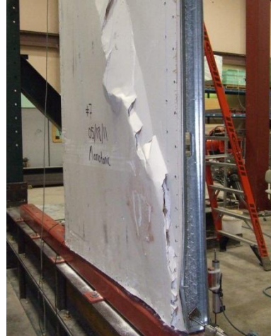
Figure 5: Gypsum board cracking and end stud distortion
