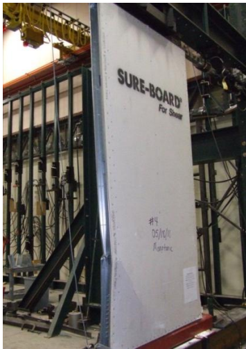
Figure 6: End stud buckling
