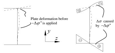
Figure 5: Plate deformation under bending and stresses caused by  $-\Delta \varphi$ "
