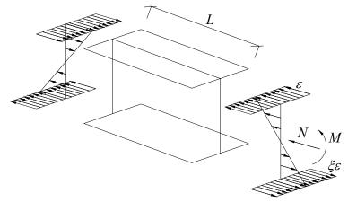
Figure 4: Load combinations defined in strain for major axis bending
