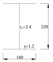
Figure 6: Geometry of the cross-section (dimensions in mm)
