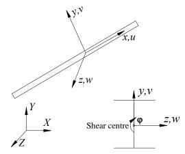
Figure 3: Coordinate axes and shear centre displacements
