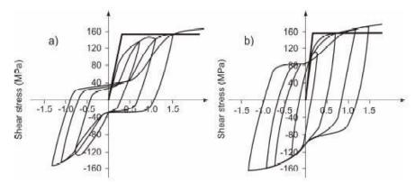
Figure 4: Hysteresis behavior of a) an unstiffened (P-2.3) and b) a heavily stiffened steel plate wall (PR-2.3-M2-60) (Takahashi et al., 1973)
