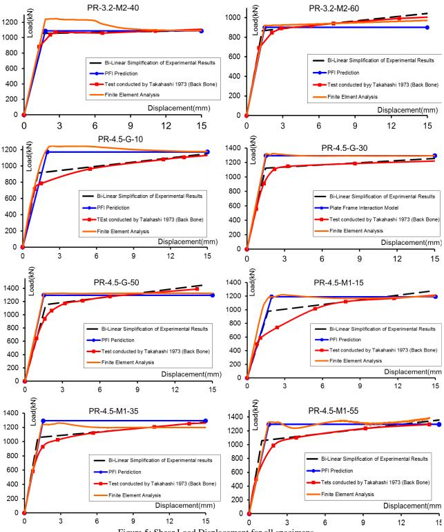
Figure 5: Shear Load Displacement for all specimens
