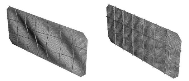
Figure 7: Buckling deformation of stiffened plate: global buckling mode (left), and local buckling mode (right)
