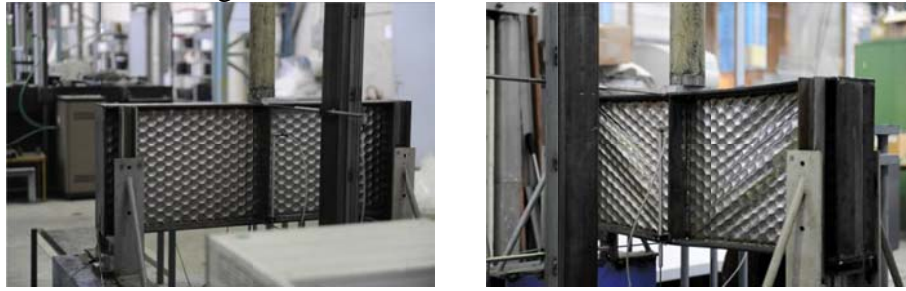
Figure 13: Test girder 4.1 during the shear load test
