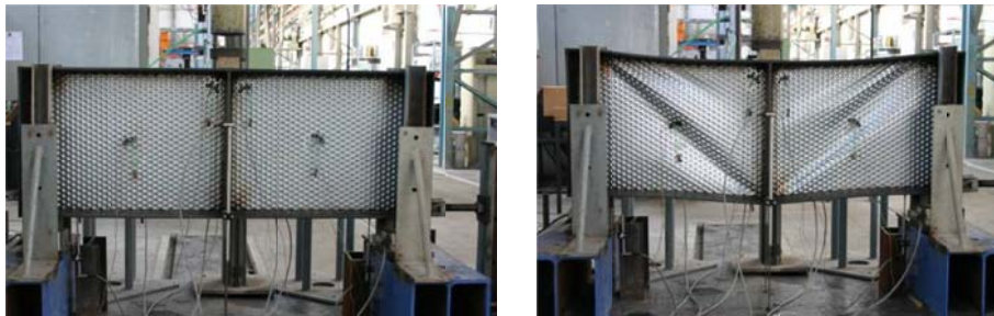
Figure 14: Test girder 6.1 during the shear load test
