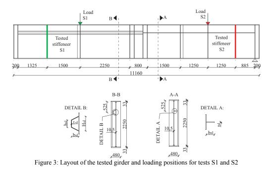
Table 1: Geometry of the tested steel plate girders Web Upper flange Longitudinal stiffener Bottom flange  $h_w$ tw а  $b_{fl}$  $b_{f2}$  $\mathrm{H}_{\mathrm{sl}}$  $h_{sl}$  $b_{sl}$  $t_{f1}$  $t_{f2}$ t<sub>sl</sub> Specimen [mm] S2 1500 7 22 320 22 90 1500 320 / 10 /
