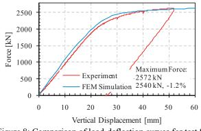
Figure 8: Comparison of load-deflection curves for test S1
