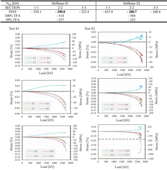
Table 2: Axial force in the transverse stiffener at maximal girder resistance, taking into account effective part of the web 15tew
