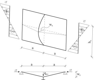
Figure 2: Calculation model for deviation forces in EN 1993-1-5
