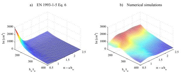
Figure 14: Required stifness of stiffener as a function of web slenderness and panel aspect ratio
