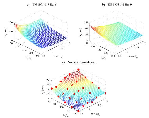
Figure 18: Size  $b_{st}$  ( $t_{st} = b_{st}/10$ ) of the flat stiffener to fulfill stifness stifness condition form Fig. 17
