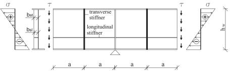
Figure 10: Numerical model of stiffened plate girder under combination of high bending moment and shear force
