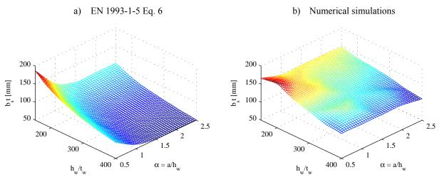
Figure 15: Size  $b_{st}$  ( $t_{st} = b_{st}$  /10) of the flat stiffener to fulfill stifness condition from Fig. 14
