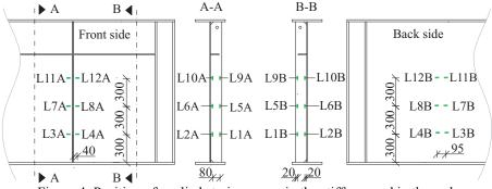
Figure 4: Position of applied strain gauges in the stiffener and in the web
