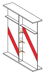
Figure 7: Cross-sections in the stiffener where the axial forces were evaluated
