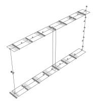
Figure 13: Numerical model of plate girder under shear force
