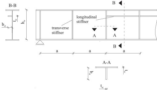
Figure 1: Notation of the stiffened panel
