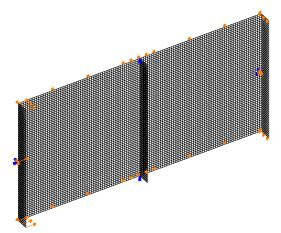
Figure 16: Numerical model of transversally stiffened plate subjected to axial force
