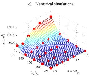
Figure 17: Required stifness of stiffener as a function of web slenderness and panel aspect ratio
