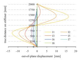
Figure 11: Out-of-plane displacement along the transverse stiffener for girder  $h_w/t_w=250$ ,  $\alpha=1$ ,  $\gamma/\gamma^*=3.0$ ,  $A_{f}/A_w=0.7$
