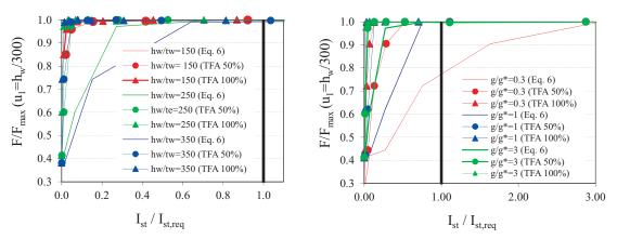
Figure 12: The normalized force obtained at out-of-plane displacement of  $h_w/300$  for different stiffness of stiffener
