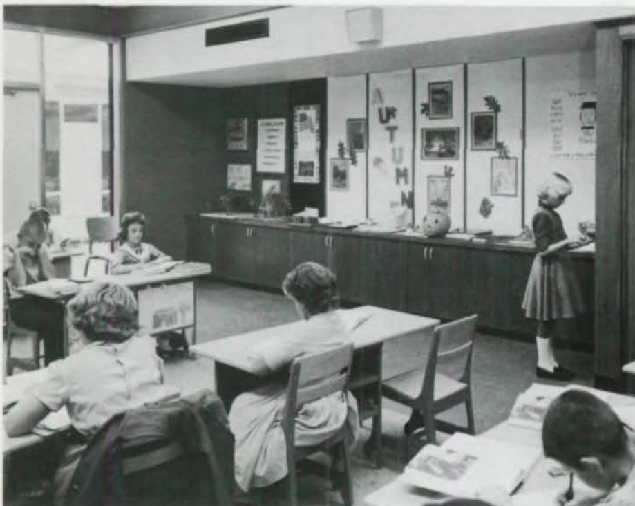
Classrooms feature gray glass to cut glare and as much tackboard and counterspace as could be provided. Ceilings are of exposed formboard and acoustical plaster.
