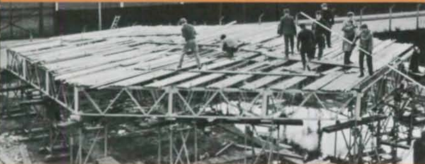
FIGURE 3. Three-way double-layer grid under test. Steel tubes have been used as the superimposed loading.
