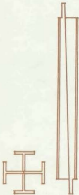
Each tapered column section is made up of four identical tee sections welded stem to stem. The tees were cut from 12WF27 sections, as illustrated.
