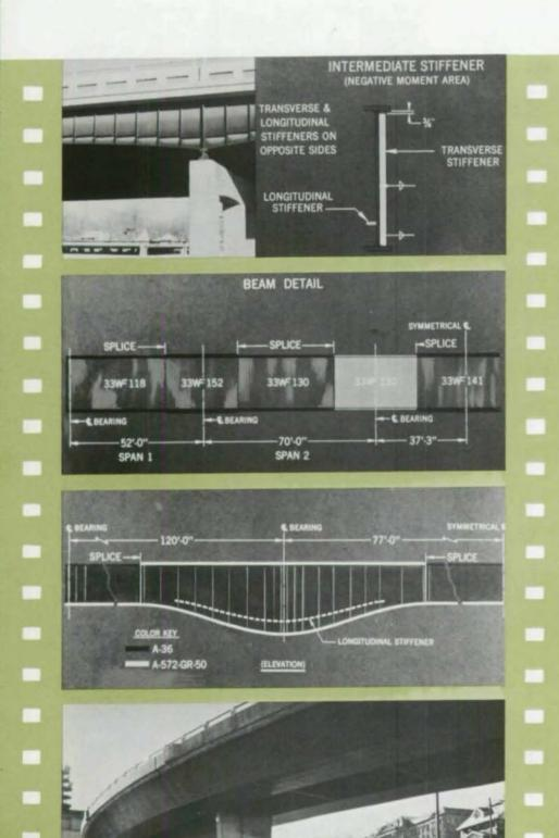
This bridge of the 50's was reinforced with longitudinal and transverse stiffeners on the same plane. This required cutting and fitting of the transverse stiffeners at points of intersection. Modern design techniques fully consider labor costs as well as those of material, and are more selective in placing steel effectively. By locating the transverse stiffener on one side of the web and the longitudinal on the other, considerable labor cost is saved.
