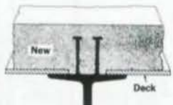
(Left) Steel decking may be laid on beams after old concrete is removed. Shear connector studs are welded and new concrete is poured.
