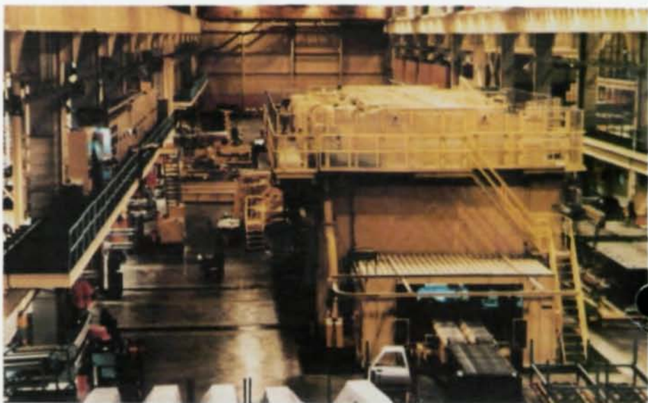
Building bay with large transfer press (above). Below, two operating press lines were installed within one wide building bay.
