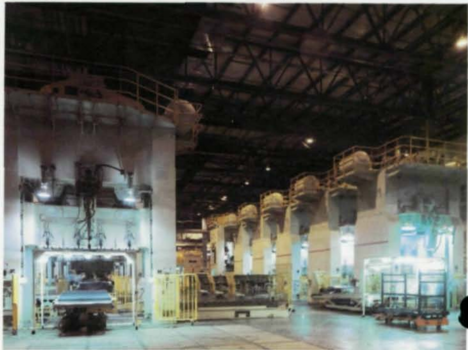
Building bay with large transfer press (above). Below, two operating press lines were installed within one wide building bay.
