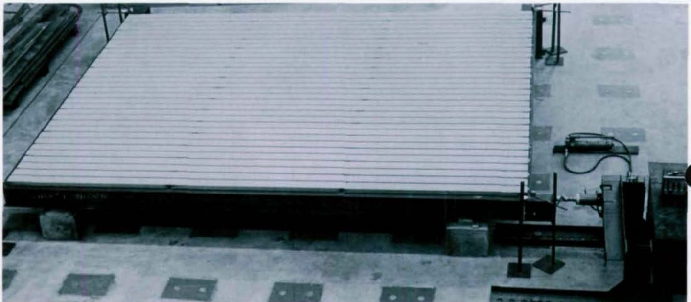
Typical test arrangement represents roof area, with specific deck type and fastening method. Far side restrained as at end wall. Measured shear forces are applied along near side and all corner movements are measured for stiffness evaluations.
