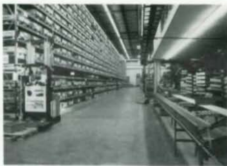
High-rise steel shelving and parts conveyor system
