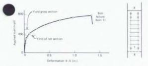
Fig. 8.2. Typical load versus deformation curve for lap joints in which restraints against bending are provided
