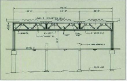
Twin 90' Warren Trusses were erected on each side of a column line during the removal of 22 large concrete columns. The trusses, which worked in pairs, supported the ceilings 300 lb. live loads on crossbracing installed between the two trusses. Photography by PHOTOtechnique
