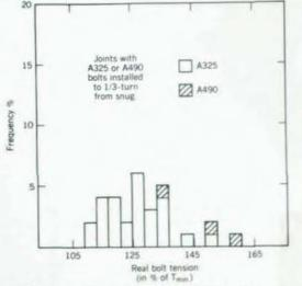
Fig. 5.8. Joints with A325 or A490 bolts installed to 1 turn from snug.
