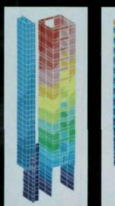
All three SCADA packages include the following elements: 3D truss, 2D and 3D beam, 3 & 4-node thin plate/shell, 3 to 9-node thick plate/shell, plane/axisymmetric, and 4 to 27-node solid.
