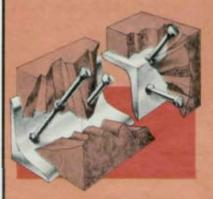
Concrete Anchoring – Stud welded headed concrete anchors deliver specified axial tension and shear strength values and can be applied up to three times faster than hand welded anchoring devices. Other advantages include much higher yield points, elimination of costly set-up time for shearing and bending, stronger welds, reduced material handling and no distortion.
