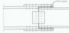
Fig. 10.1. Beam or girder splice with filler plates.
