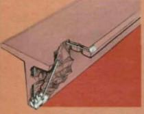
Precast/Prestressed – Because of their known values, anchor studs can be used in standardized designs for such connections as bearing plates for beams and tees, shear keys for tees, column baseplates, and various other embedded steel elements. In these applications, stud welding reduces cost per plate, ensures consistently high weld quality, frees certified welders for other jobs, eliminates long lead time and storage problems.
