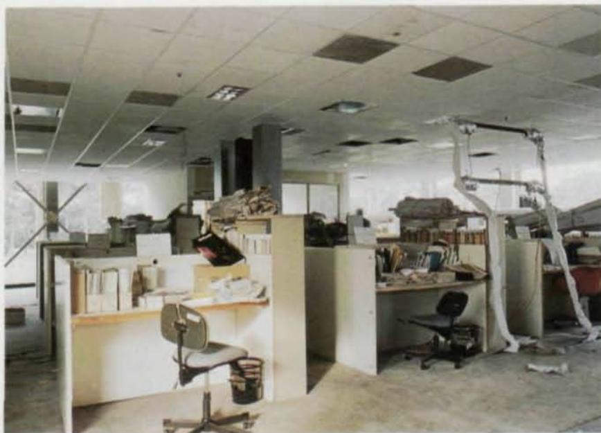
The interior of the test structure was set up to closely resemble actual office conditions, including modular furniture and piles upon piles of papers, files, and other miscellaneous combustible items.
