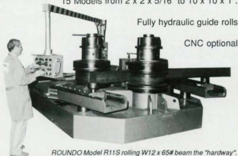
ROUND Model R11S rolling W12 x 65# beam the "hardway".
