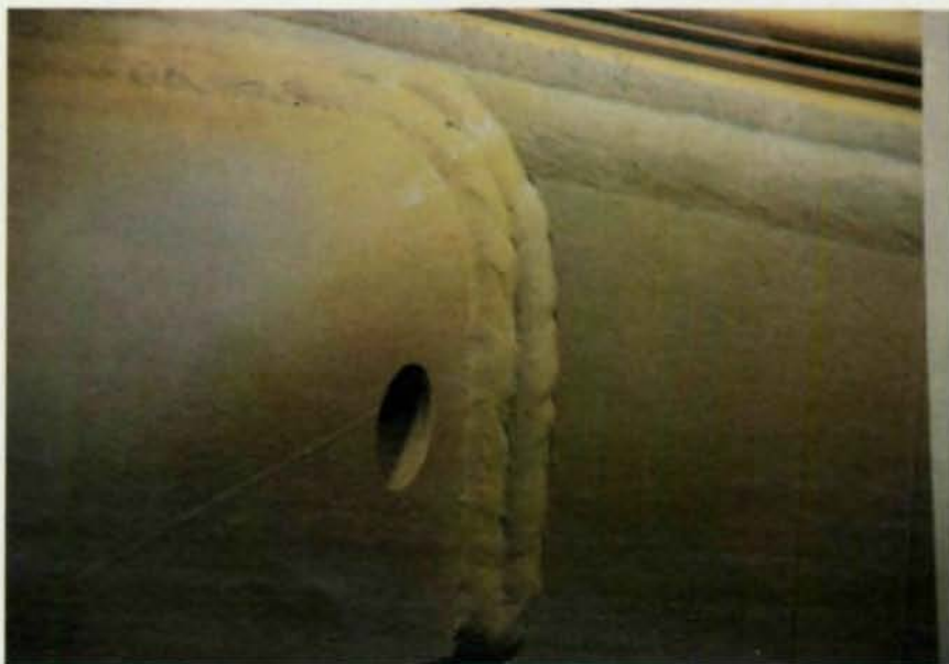
No further preparation is needed for a machine weld (photo courtesy of Lincoln Electric).
