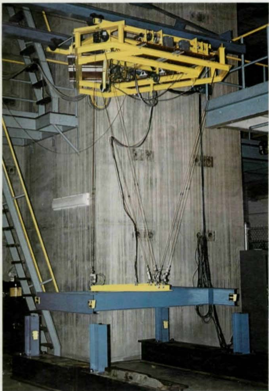
ATLSS Center's multi-directional testing facility is capable of testing full-scaled structural specimens in any direction or directions.
