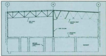
The renovation included built-in-place trusses spanning from the south wall to the support columns. The transfer truss supported the intermediate north truss ends, and joists spanned between the new north/south trusses.
