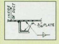
required spacing not exceeding the calculated  $L_{\rm u}$  for the effective section. The suggested lateral support detail is shown.
