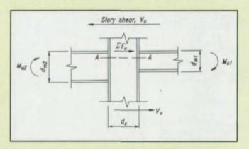
In checking panel zone web shear in a column member why is M<sub>1</sub> defined as the sum of the lateral load and gravity load moments on the leeward side of the connection, and M<sub>2</sub> defined as the difference between the lateral load and gravity load moments on the windward side of the connection? It seems to us that the difference of moments apply on the leeward side and that the sum of the moments should apply on the windward side.
