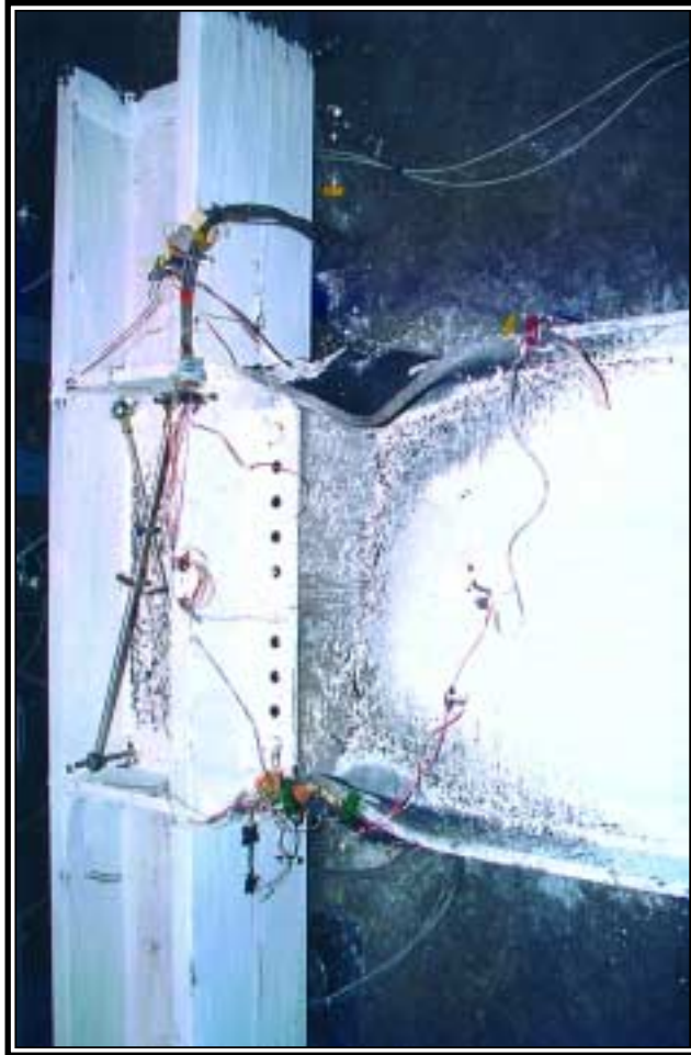
Figure 2: Beam yielding and buckling of Specimen A-4 (E70TG-K2 electrode)
