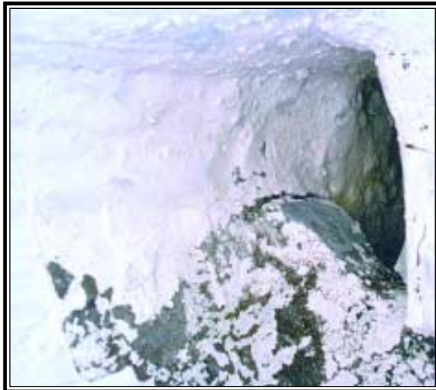
Figure 3: Stable crack at access hole of Specimen A-4 after large rota- tion
