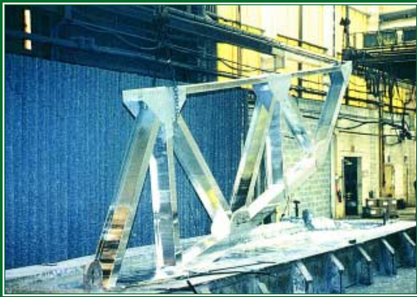
Pictured is a truss member as it is dipped in a galvanizing bath.
