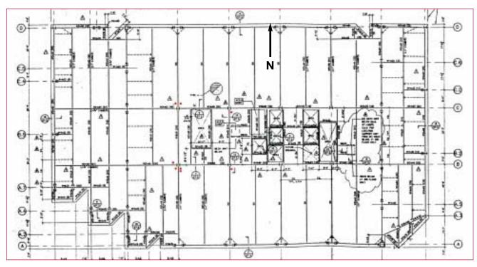
Figure 1: Fifth floor framing (red dots indicate de-torquing noise events)
