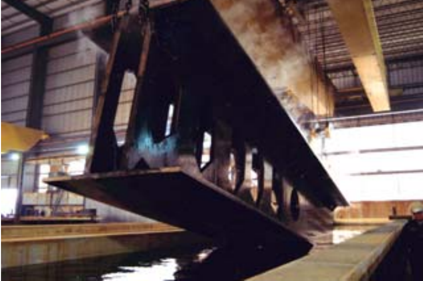
In January 2003, A-Plus Galvanizing, Inc., in Salina, KS dipped what might have been the heaviest piece of steel ever galvanized in the world—an 86,000-lb. bridge tower anchor. Photo credit: John Gregory at Arrow Printing Company, Salina, KS.
