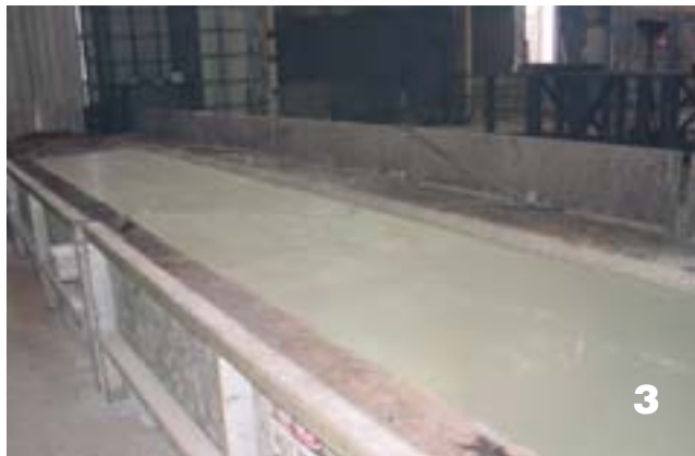
AAA Galvanizing's 51' x 6'8" x 9'3" galvanizing kettle, filled with molten zinc heated to approximately 850°F.
