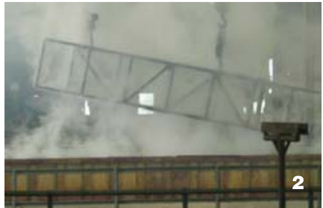
Steel exits the flux tank after being bathed in a solution of zinc ammonium chloride. The flux heats and coats the steel to prevent it from oxidizing.
