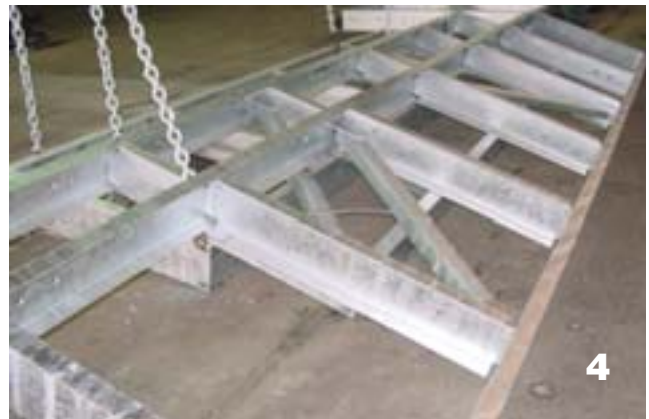
Galvanized steel, cooling after immersion.
