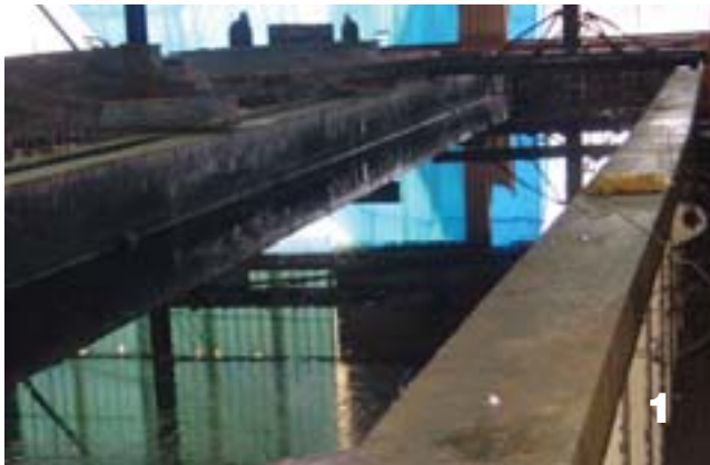
First step: organic material is removed by dipping steel in a hot caustic bath.
