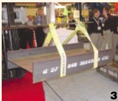
The scrap was melted and rolled into a wide-flange, which returned to Baltimore...
