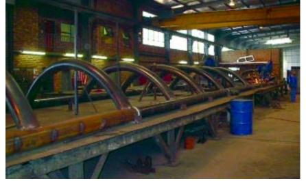
Curved, round HSS segments were welded to the stringers in the shop to form half-shells (the sides of the bridge). To create a complete spiral, more curved, round HSS segments were welded between the left and right half-shells.
