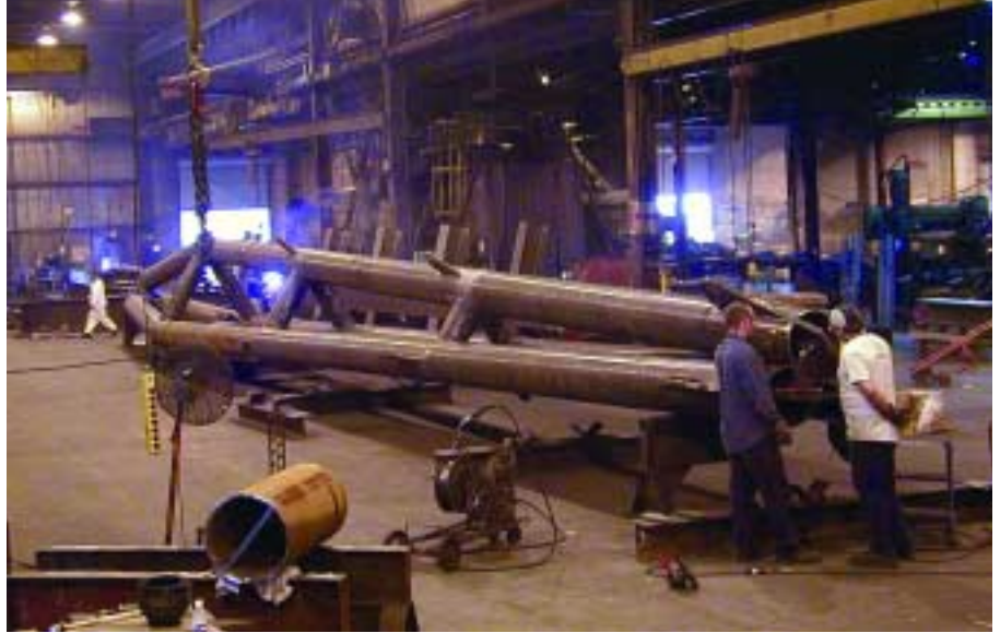
Above, left and right: The 10-story-tall masts are composed of three 18"-diameter steel hollow structural sections (HSS) arranged in a triangular, tapering form, and tied together with 12.75" HSS
