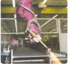
The Kaltenbach KC1200 robotic coping machine (2003 Hot Product Honorable Mention) is one of a number of robotic fabrication machines that recently have been introduced to the steel-fabrication industry. Jesse Engineering's Robotic Series SHC-BC-R (next page) also uses a robot to precision-cut structural steel members.
