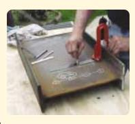
for erectors, because when things don't line up, the job cannot be completed on schedule, and everyone is thrown off track. The beam gauge tool helps prevent this problem.
