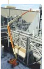
the majority of the work envelope is a restricted 1,000 lb (unrestricted is 500 lb). The machine includes JLG's QuikStik® boom that allows the platform to be lowered to the ground while the tower boom is fully extended. With this feature, workers can go from ground level to full elevation in 115 seconds. A standard feature of the Model 1250AJP is the SkyPower™ package, which includes a 7,500-watt generator that provides power to welders and other platform-mounted accessories.
