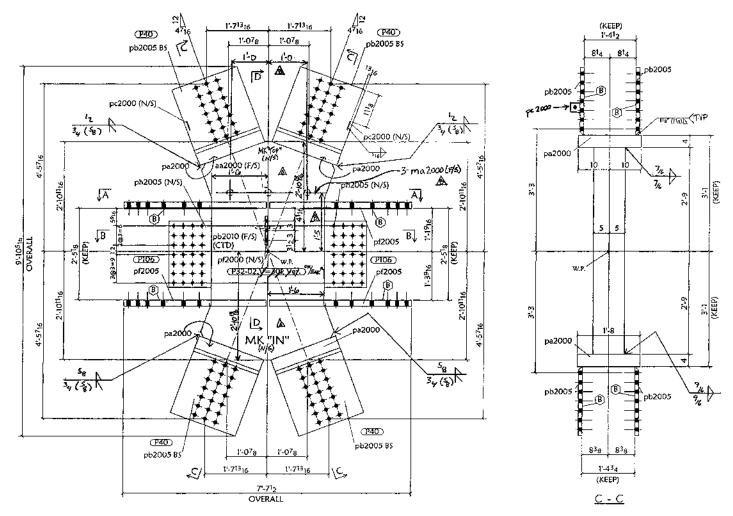
This detail shows a typical node for the building. Eighty-four similar pieces were fabricated from 10"-thick machined steel plates.
