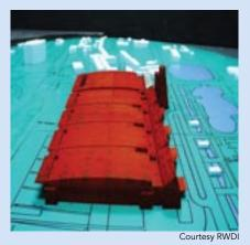
design wind loads from measurements taken from more than 700 pressure taps at the model surface.
