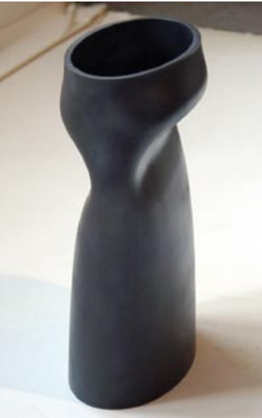
This test sample of an EHS failed by local buckling.
