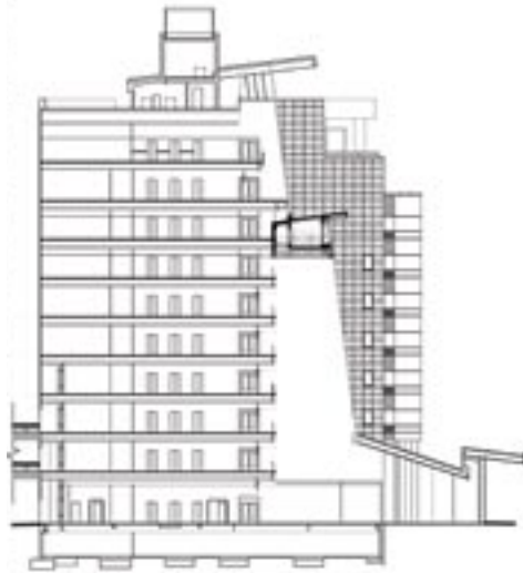
The seven-story atrium extends from the ground floor up to a mechanical space.
