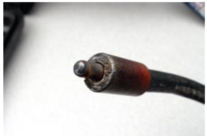
Caused by slow travel speed or holding the tip too close to the weld, burnback requires the contact tip to be replaced.
