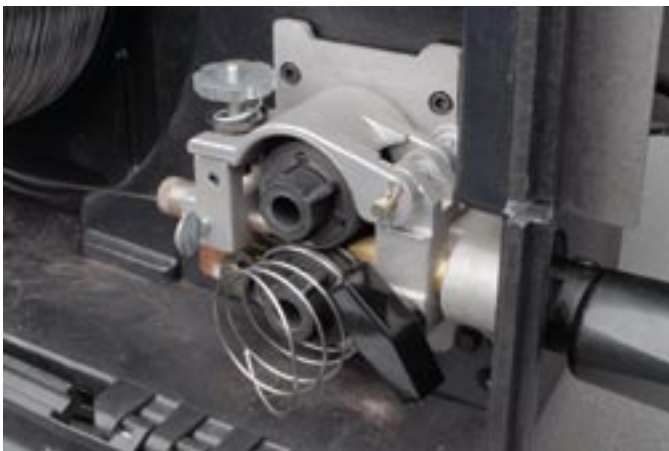
Often resulting from incorrect drive roll tension, birdnesting, as seen here, can be a frustrating source of downtime.
