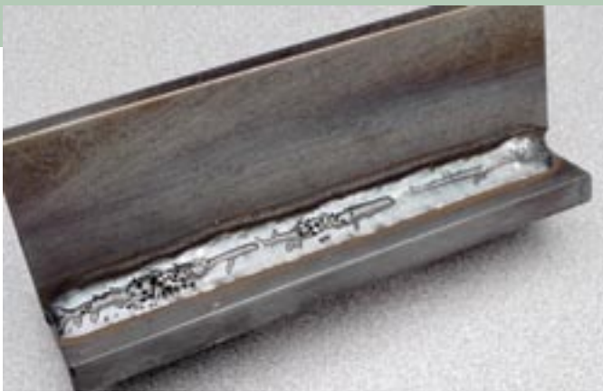
This image shows a combination of worm tracking and porosity, both outcomes of too much voltage. Worm tracking is both easily diagnosed and easily corrected by lowering your voltage. Porosity, seen on the face and cross section of this weld, can significantly weaken the structural integrity of the weld.
