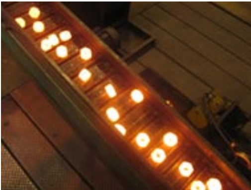
Nuts, still orange-hot, after being formed.
