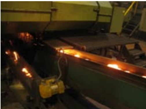
Punch-outs (left, in photo) are recycled.
