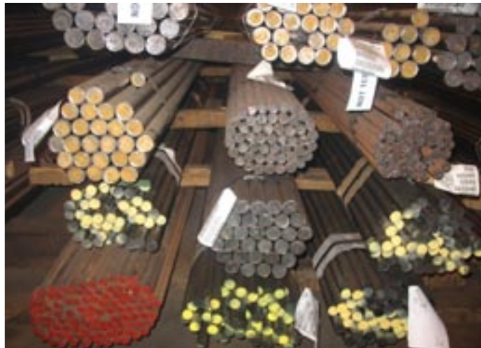
The ends of the bars are color-coded by grade.
