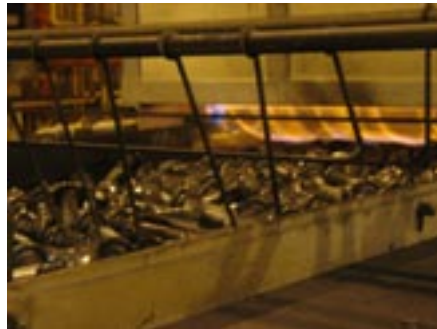
Hardening involves temps of up to 1,570 °F.
