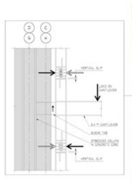
A detail of the connection between the Vierendeel exterior framing and a concrete core.
